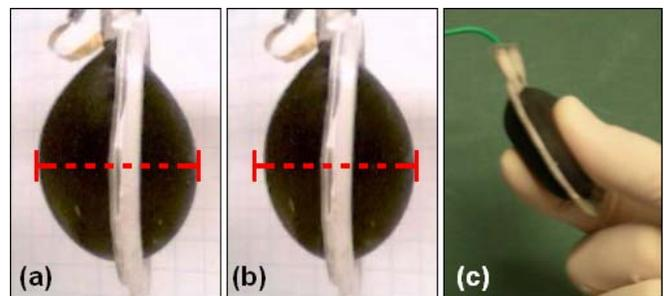
**Figure 9:** Silicone-made prototype display of cardiac chamber contractility: (a, b) contractility due to an electrical driving of the left-side membrane (the dashed segment can be used for comparison); (c) palpation of the prototype.
