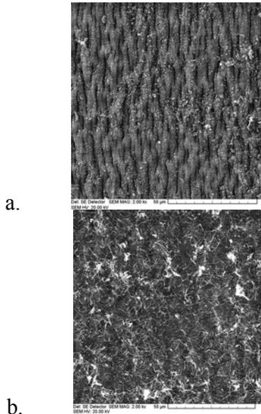
**Figure 20:** SEM image of conducting thin film compliant electrodes deposited on acrylic pressure sensitive adhesive VHB elastomer (0,25 mm thick) after 2000 uni-axial stretch-relax cycles:
