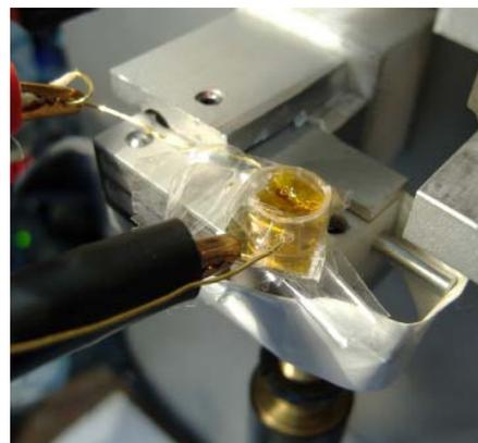
**Figure 16:** PFS polyanion hydrogel during a cyclic voltammetry test.
