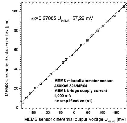
**Figure 18:** MEMS cantilever displacement microsensor:
