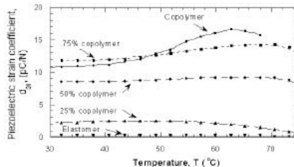
**FIGURE 10:** The temperature dependence of the piezoelectric strain coefficient,  $d_{31}$ , of the blend films (1 Hz) as a function of the various compositions.
