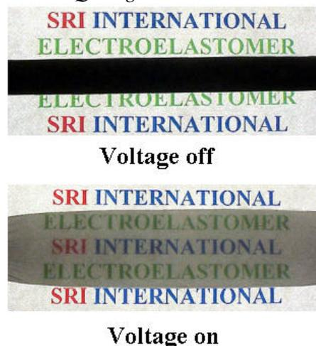
**Figure 12:** Opacity variation of an acrylic-based dielectric elastomer film due to an applied voltage.
