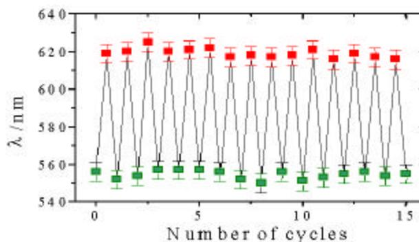
**FIGURE 4:** Reversibility of the helix “untwisting – twisting” process under the UV-irradiation and heating of the polymer film.
