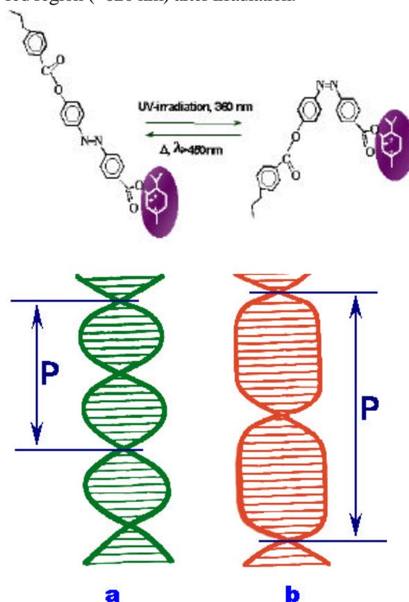
**FIGURE 3:** Scheme of cholesteric helix (a) before the irradiation and (b) untwisting of the cholesteric helix after UV-irradiation of polymer film.
