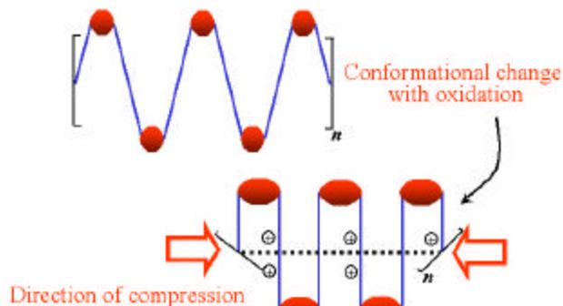
**FIGURE 9:** Actuator contraction mechanism.
