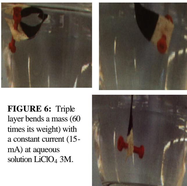
**FIGURE 6:** Triple layer bends a mass (60 times its weight) with a constant current (15-mA) at aqueous solution LiClO<sub>4</sub> 3M.
