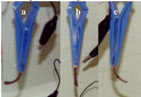
**FIGURE 1:** Movement of 'Shell type' actuator in air based on polyaniline films References
