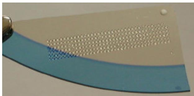
**FIGURE 13:** Printed gels on the platinum board, (dots are 100 microns apart).
