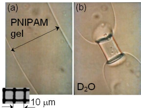
**FIGURE 2:** Micro-video image of Poly(*N*-isopropylacrylamide) (PNIPAM) gel rod in D<sub>2</sub>O before (a) and after (b) illumination by 0.75 W power laser illumination at  $\lambda = 1064$  nm wavelength.
