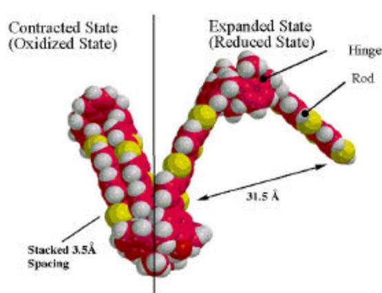
**FIGURE 8:** Chemical structure of a candidate molecular actuator.
