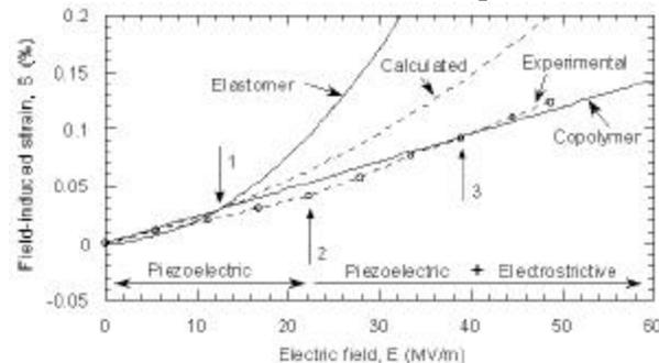
**FIGURE 11:** Comparison between the experimental strain response of the 75 wt.% copolymer blend with the prediction
