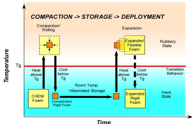
**FIGURE 5:** CHEM processing cycle
