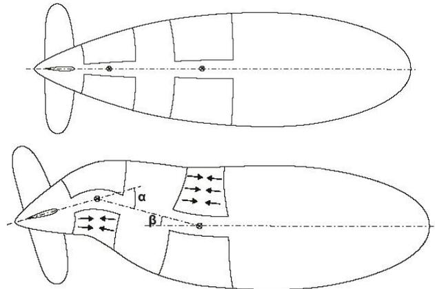
FIGURE 8: A graphic view of the envisioned EAP activated blimp.
