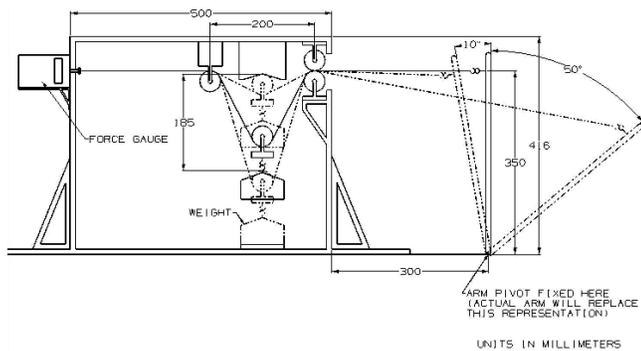
**FIGURE 3:** The competing arms testing fixture (see larger drawing on <http://ndea.jpl.nasa.gov/nasa-nde/lommas/eap/EAP-armwrestling.htm>).
