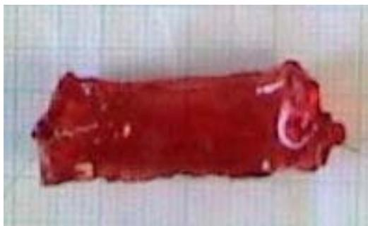
**FIGURE 5:** Electroresponsive smart material with embedded electrodes. Red dye has been added to enhance visualization.
