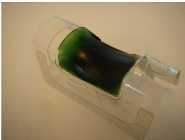
**FIGURE 10:** Soft frame actuator prototype with PANi-elastomer electrodes.
