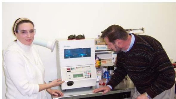
**FIGURE 6:** Lew Meixler and Lenore Rasmussen at Ras Labs with UV photocuring equipment used in the production of electroresponsive gels.
