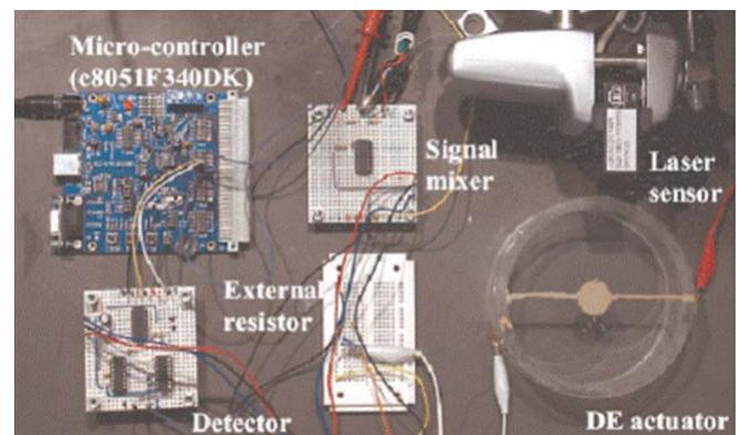
**FIGURE 2:** Dielectric elastomer (DE) actuator and sensor.
