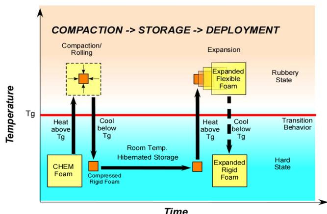
**FIGURE 11:** CHEM processing cycle
