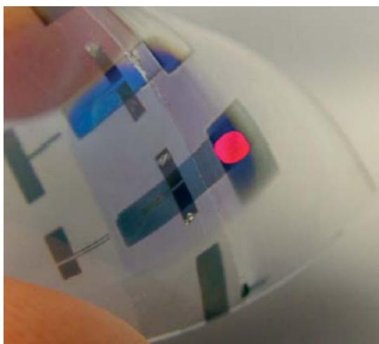
**FIGURE 8:** Operation of a flexible optothermal switch, based on pyroelectric copolymers of vinylidene fluoride and trifluoroethylene and - voltage organic field-effect transistors.
