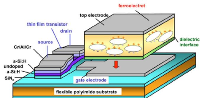
**FIGURE 7:** Concept of the “ferroelectret field-effect transistor”. The voltage generated by the ferroelectret upon touching the element, or by means of acoustical waves controls the current through the flexible field-effect transistor.
