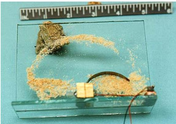
Surface wiper removing dust from a glass window using Perfluorinated Ion-exchange membrane platinum.
