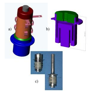
Figure 4. A Solidworks assembly drawing of the (a) folded horn, piezoelectric stack actuator, and backing. (b) Cross section of the folded horn. c) A photograph of assembled folded horn compared to standard stepped horn.
