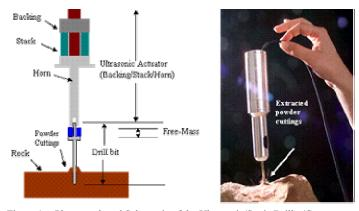
Figure 1. Photograph and Schematic of the Ultrasonic/Sonic Driller/Corer.
