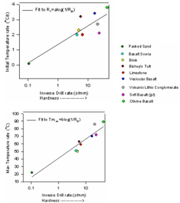
**Fig. 2:** The measured temperature maxima and initial temperature rate as a function of hardness (inverse drilling rate) for variety of media.
