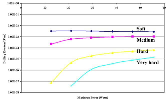
**Fig. 3:** Analytical drilling rates in rocks with various hardness levels using 10W average power. The rocks are classified by their compression strength, where: Soft: 0 – 50; Medium: 50 – 100; Hard: 100 – 200; and Very hard: >200 (MPa).
