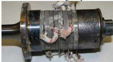
**Figure 8:** Photograph of the first HT USDC actuator breadboard. The piezoelectric stack was made of LiNbO<sub>3</sub> and was tested at 500°C.
