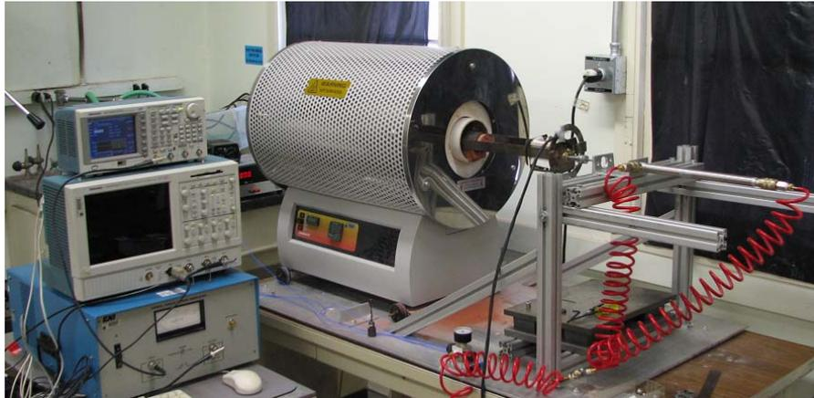
**Figure 3:** The high temperature testbed setup including the instrumented chamber, the support of the sampler (with the sampler and sample), the pneumatic pushing setup as well as the drive and measurement instruments.
