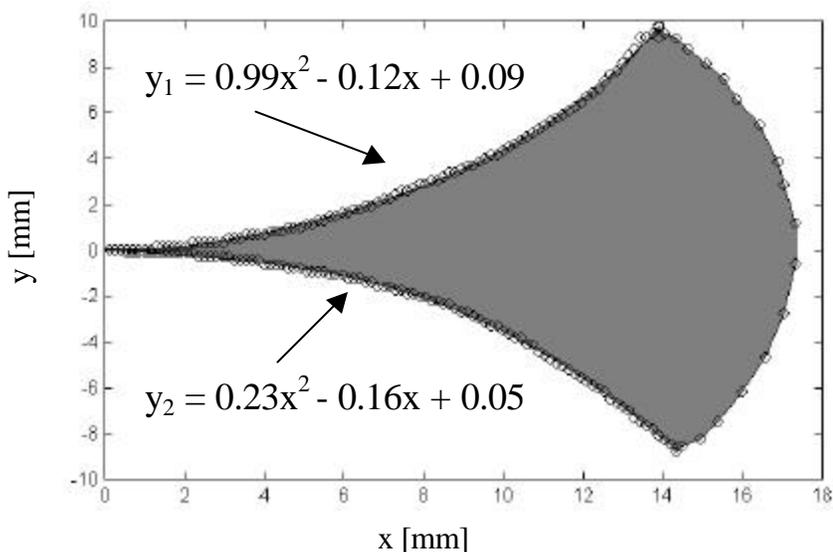
Figure 2. Bending response of Nafion to applied voltage of 3.0V, 0.05 Hz. The shaded region represents the swept area equal to  $125\text{mm}^2$ .
