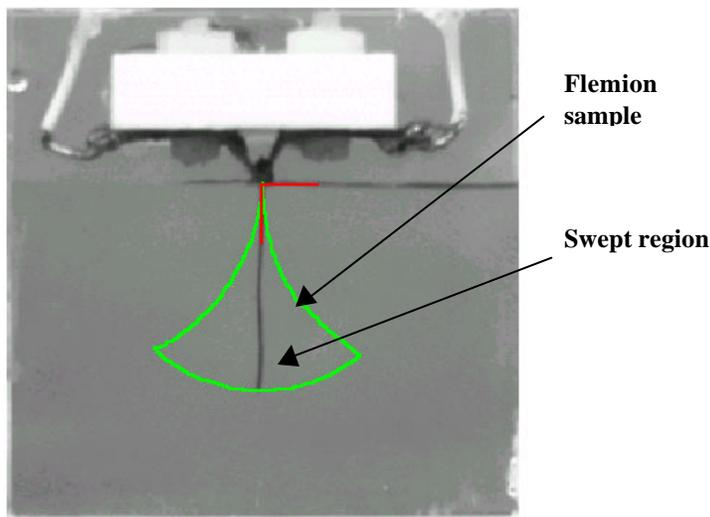
Figure 1. Image displaying electrically induced bending deformation of Flemion sample.
