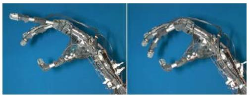
**FIGURE 9:** Robotic hand (Photographed at JPL) is available at JPL as a platform for demonstration of EAP actuators [Courtesy of Dr. Graham Whiteley, Sheffield Hallam U., UK. The actuators were installed by Giovanni Pioggia – University of Pisa, Italy/JPL].
