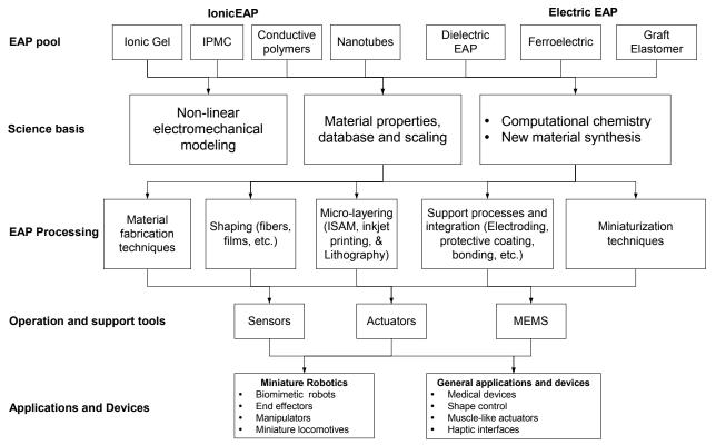
FIGURE 6: EAP infrastructure block diagram
