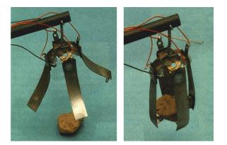
FIGURE 3: 4-finger EAP gripper lifting a rock
