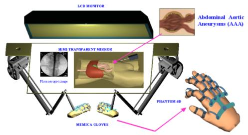
**FIGURE 10:** Performing virtual reality medical tasks via the Electro-Rheological Fluid based MEMICA haptic interface offers the potential of highly attractive interactive simulation system.
