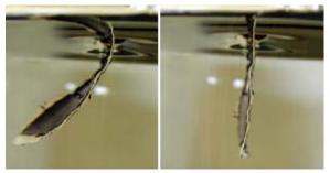
**FIGURE 5**: Conductive EAP actuator is shown bending under stimulation of 2-V, 50-A.
