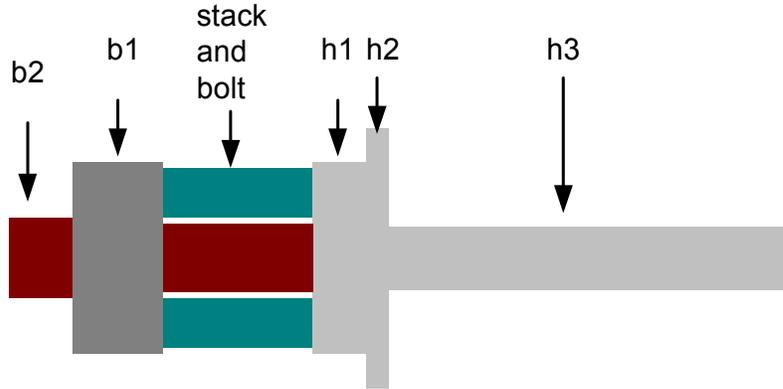
**Figure 1.** A standard stepped horn (three steps)
