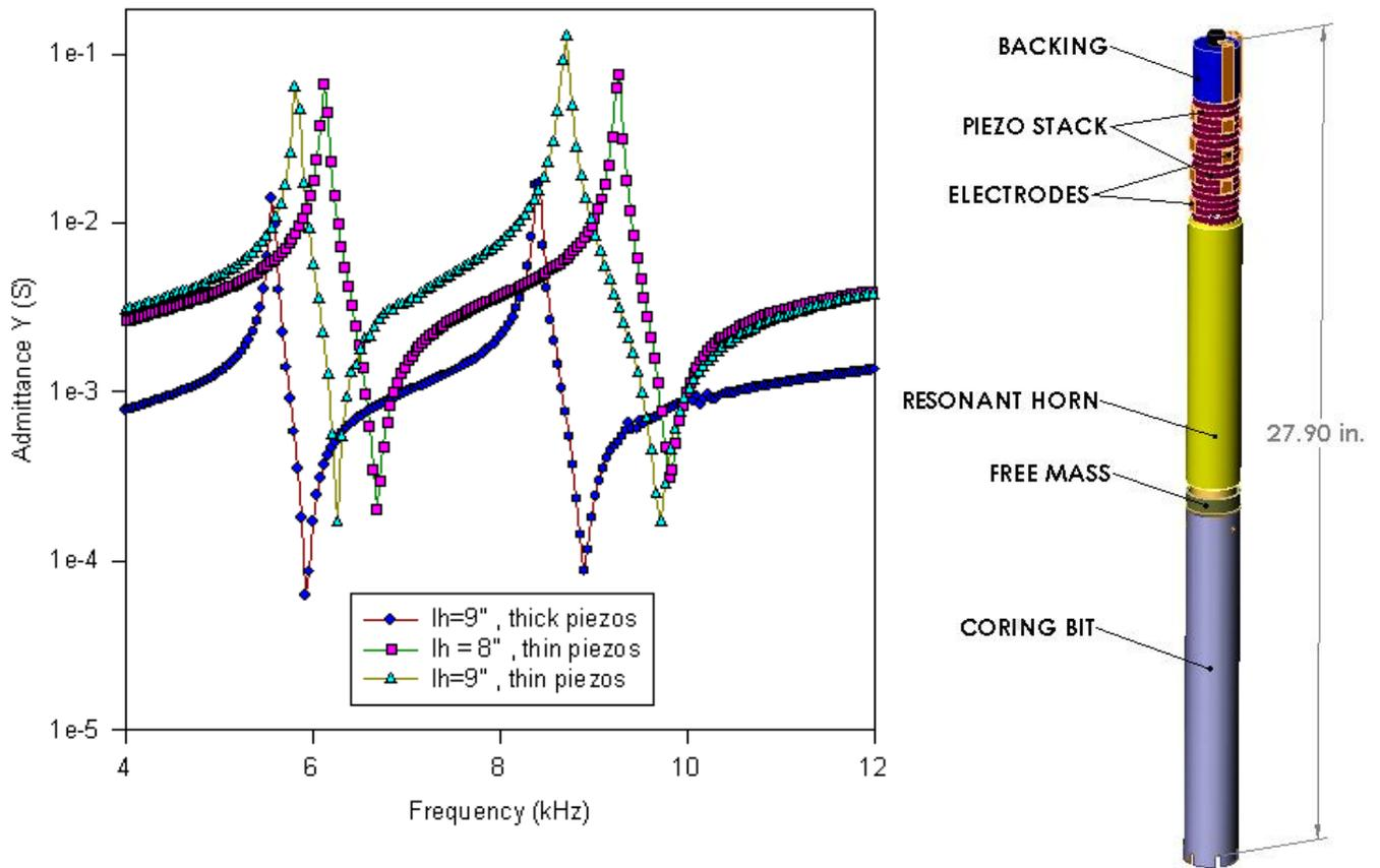
**Figure 11.** The impedance spectra of the large inverted horns designed for the ultrasonic gopher shown to the right. By adjusting the piezoelectric thickness and reducing the horn length we were able to adjust the baseline impedance, the resonance frequency and the impedance at resonance. The latter is useful with regards to impedance matching of the driver and the device.
