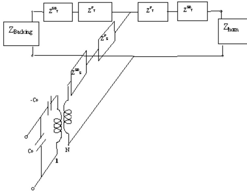
**Figure 2.** Mason's equivalent circuit for a piezoelectric ring stack with a center stress bolt. Parameters of the model can be found in earlier work<sup>6,9</sup> Excellent agreement between the full model and experimental results were reported.
