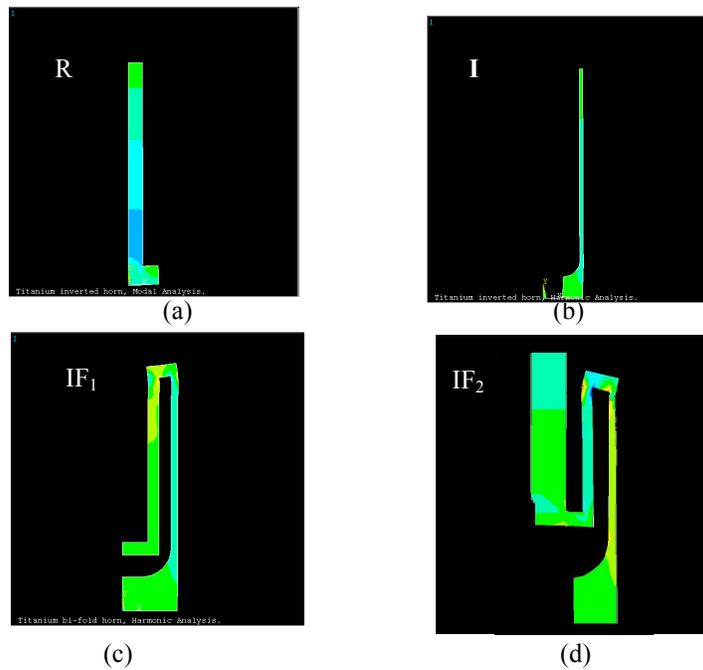
**Figure 6.** ANSYS axis-symmetric mesh of the a) regular stepped horn R, b) inverted stepped horn IF<sub>0</sub>, c) inverted stepped horn with 1 fold IF<sub>1</sub> and d) the inverted stepped horn with 2 folds IF<sub>2</sub>.
