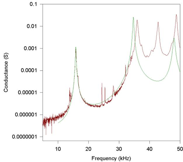
**Figure 9.** The impedance spectra of the folded horn compared to the standard model. In order to match the amplitude of the fundamental peak the quality of the horn material had to be reduced by a factor of 10. The reduced resonance amplitude in the impedance values for the folded horn is the result of the lower Q of the device, which is likely caused by poor energy transfer across the screw threads in the base.
