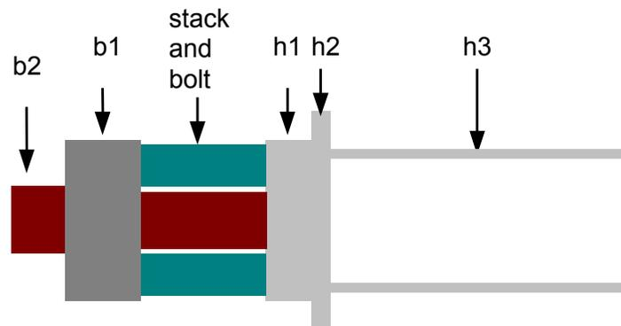
**Figure 3.** An inverted stepped horn (three steps)
