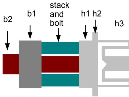
**Figure 4.** A schematic of a folded horn (2 folds)
