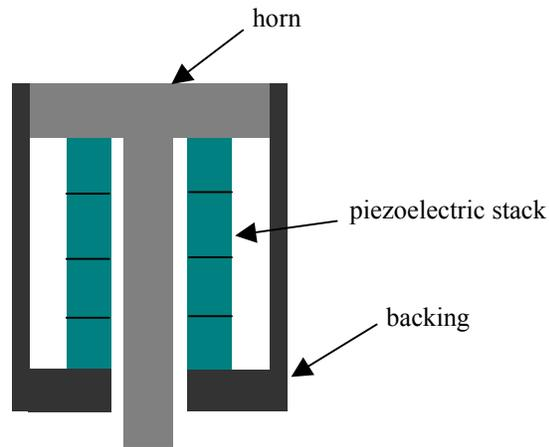
**Figure 5.** A schematic drawing of a flipped horn. The piezoelectric stack is concentric with the horn tip and generates a stress at the top surface of the horn base. The stress bolt is external and can be configured to modify the resonance frequency.
