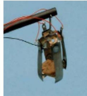
**FIGURE 2:** 4-finger EAP gripper lifting a rock.
