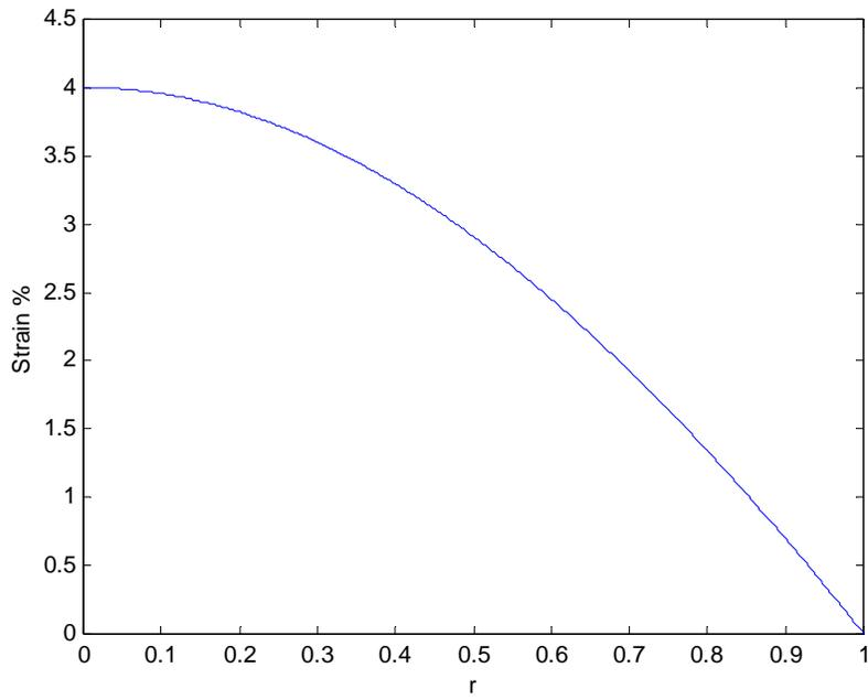
**Figure 2.** Required extension strain to form the parabolic mirror with  $z = 0.2 r^2$  from a planar sheet.
