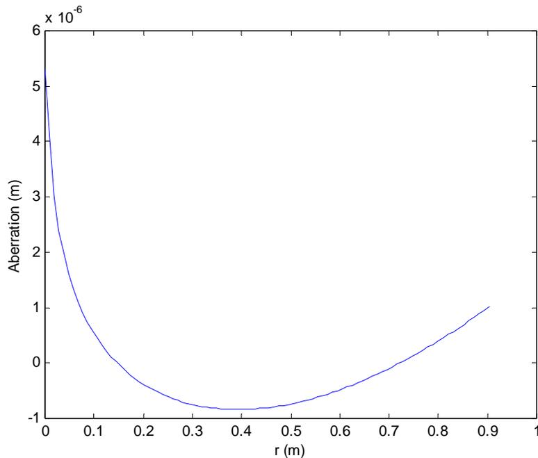
**Figure 6.** Aberration of the FEM results from the paraboloid, film thickness = 10  $\mu\text{m}$ .
