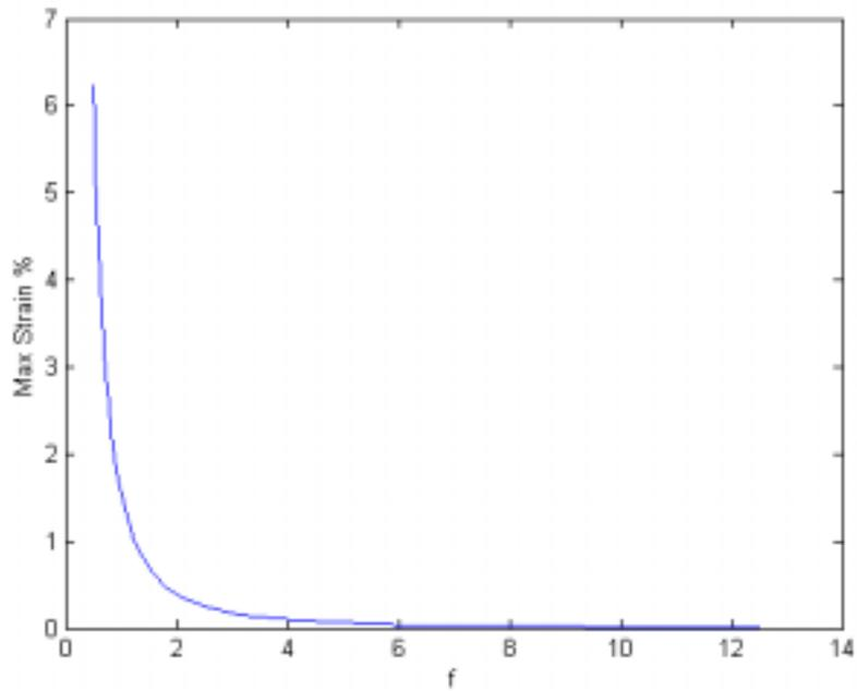
**Figure 3.** Maximum required extension strain as function of f-number of the parabolic mirror formed from a planar sheet.
