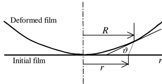
**Figure 1.** Paraboloid surface deformed from a planar disk.
