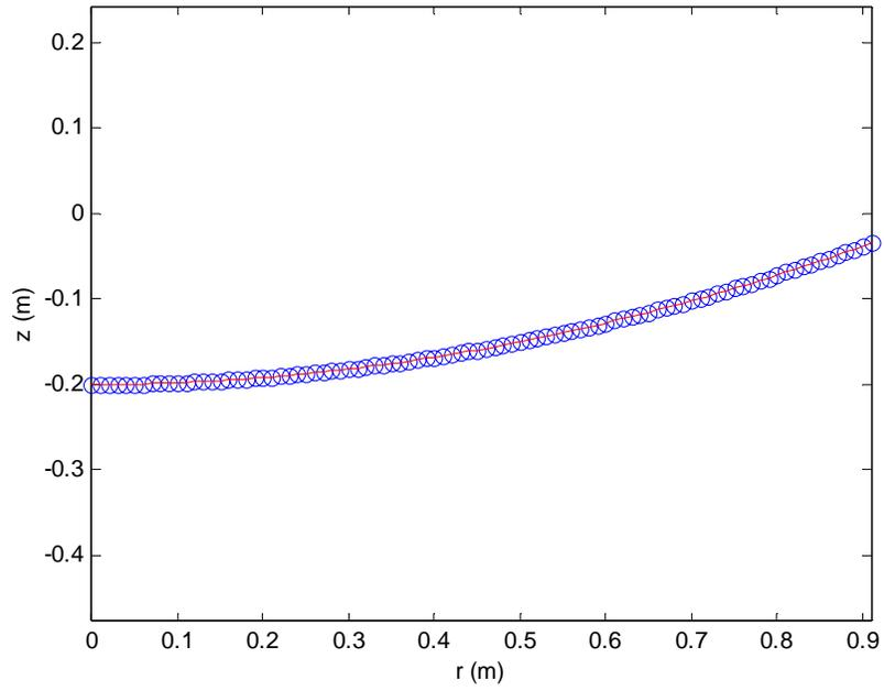
**Figure 4.** Deformed shape computed by FEM model (circle) and fitted curve of  $z = ar^2 + b$  (line).
