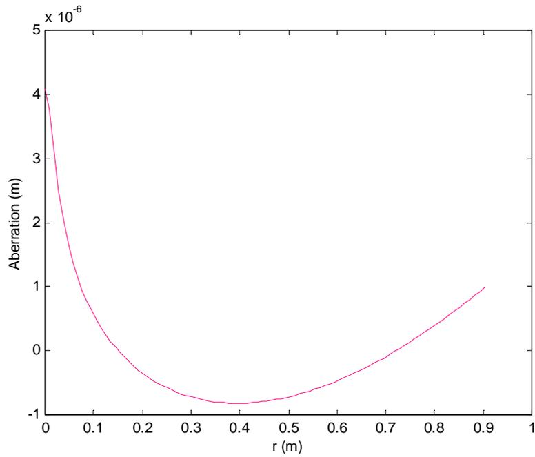
**Figure 5.** Aberration of the FEM results from the paraboloid, film thickness = 100  $\mu\text{m}$ .
