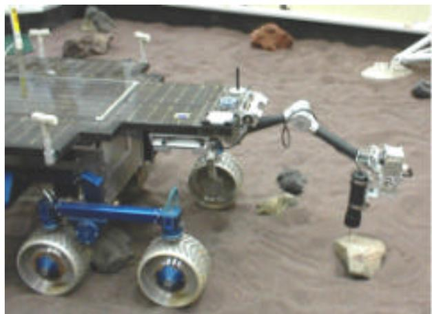
**Fig. 19.** The USDC is shown drilling while mounted on the robotic arm of the FIDO Rover.
