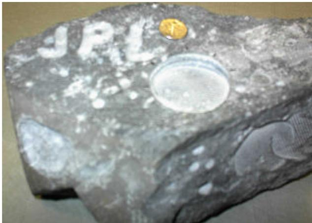
**Fig. 17.** Basalt rock sample tested using the abrasion tools shown in Fig. 17.
