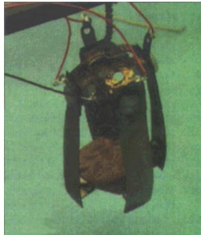
Robotic arm opens and closes a four-finger gripper composed of EAP actuators that can lift or drop objects.
