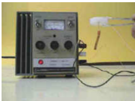
FIGURE 16: Muscle actuator synthesized by ESA process, working in air.
