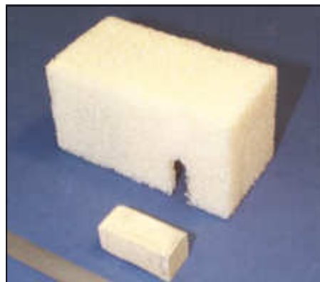
FIGURE 9: Stowed and deployed CHEM structures.
