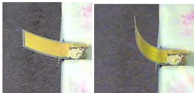
FIGURE 11: Left - The bimorph with no voltage applied to it. Right - The same bimorph after the voltage was turned on.
