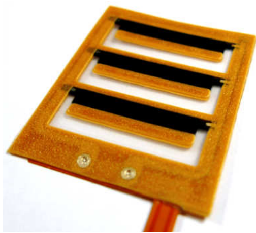
Figure 3: AMI's printed EAP actuator for haptic feedback applications
