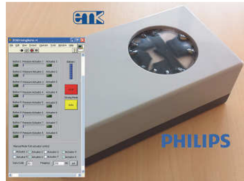
Figure 10: Handheld haptic user interface with localized tactile feedback
