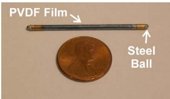
**Figure 5:** Example of electrostrictive PVDF terpolymer core-free tube actuator that generates 1 mm displacement at the tip with more than 1 N force.
