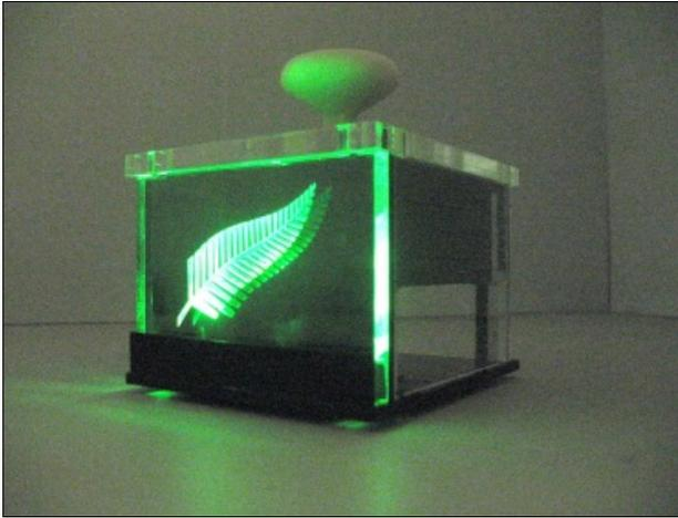
c. The four channel Artificial Muscle Control Unit: This stand-alone portable laboratory instrument simplifies the generation and control of high voltages for artificial muscle research. Features include 4 independent output channels, computer control, battery operation, and safety features that make it suitable for bench-top use.
