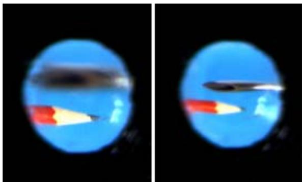
**Figure 8:** The bioinspired tunable lens in action. Electrically controlled focalization of a pencil and a syringe needle, respectively located 10 and 3 cm far from the lens.
