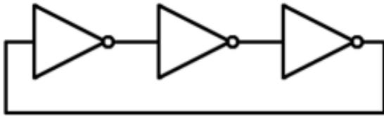
**Figure 3:** Simple three stage ring oscillator. As the number of inverters is odd the ring is unstable and will oscillate as fast as the components allow.
