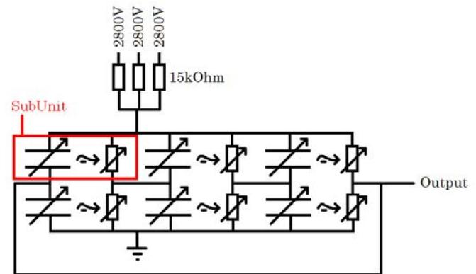
**Figure 5:** Ring oscillator design. Each pair of subunits forms an inverter, and the three inverters are connected in a ring. A WYE configuration connects three separate channels of the power supply to provide enough current.
