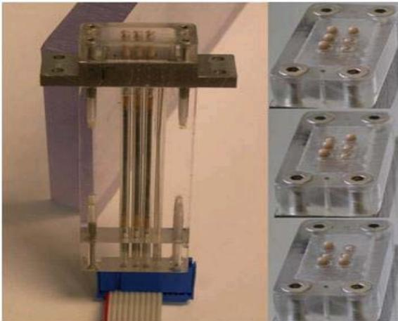
**Figure 6:** (Left) A Braille cell with 6 EAP pins which are about 3 cm long and 1.8 mm in diameter; (right) Braille pin movements when voltages are applied to different Braille pin actuators.
