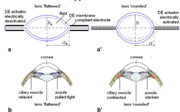
**Figure 7:** Functional analogy between the bioinspired lens and the human lens. a,b, Schematic sectional views (not in scale) of the two systems in the rest state. a',b', Corresponding views in an activation state. The annular DE actuator works as an artificial muscle, functionally analogous to the combined ciliary muscle and zonule; it radially stretches and relaxes the lens, so as to change the radius of curvature.
