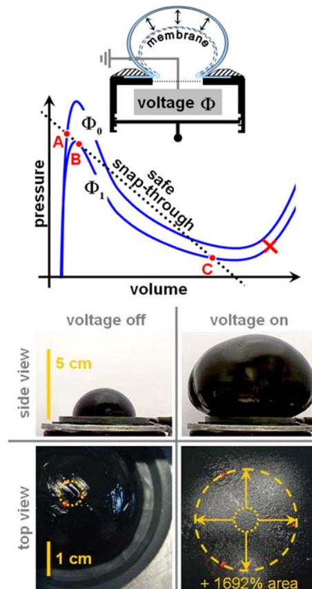
**Figure 4:** A soft dielectric membrane was mounted on a chamber of a suitable volume, pressurize the membrane into a state near the verge of the snap-through instability, and apply a voltage to trigger
