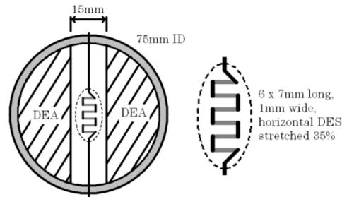
**Figure 4:** Oscillator Subunit. The two DEA compress the central DES when activated.
