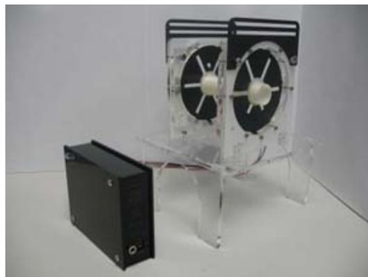
b. A hand-held dielectric elastomer generator: DE can be used to extract useful low voltage power from human movement. This will be demonstrated using a device that can be held in one hand
