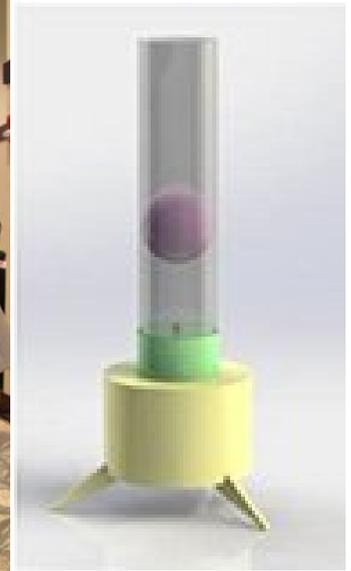
This demonstrator shows the use of circular out-of-plane dielectric elastomer actuators (COP-DEA) in a pneumatic pump application. The presented concept allows building very small and lightweight pumps. It is related to the paper with the title “Design of a dielectric elastomer actuator driven pneumatic pump”.
