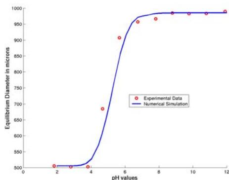
**FIGURE 13:** Equilibrium swelling of a  $400 \mu\text{m}$  hydrogel
