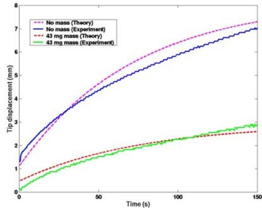
**FIGURE 11:** Experimental and analytical data for the Flemion base IPMC samples with and without tip mass.
