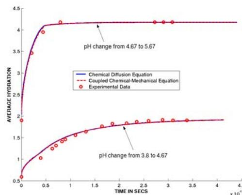
**FIGURE 14:** Swelling kinetics of a  $400 \mu\text{m}$  hydrogel for pH changes of 3.8 to 4.67 and 4.67 to 5.67.
