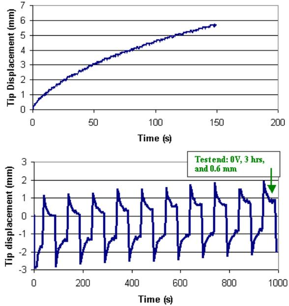
**FIGURE 10:** Displacement of IPMC as a function of time under 1-V for samples made of the following backbones: Top -Flemion (ONRI, Japan); Bottom – Nafion (ERI)
