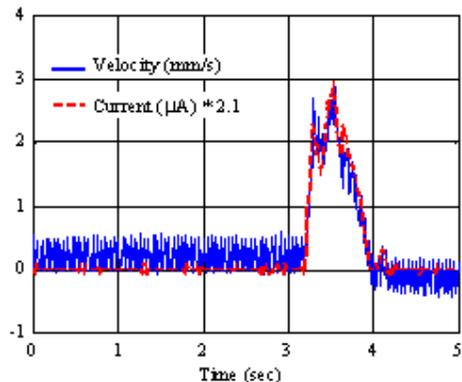
**FIGURE 15:** Velocity and current measurement demonstrating the proportionality of the two variables.
