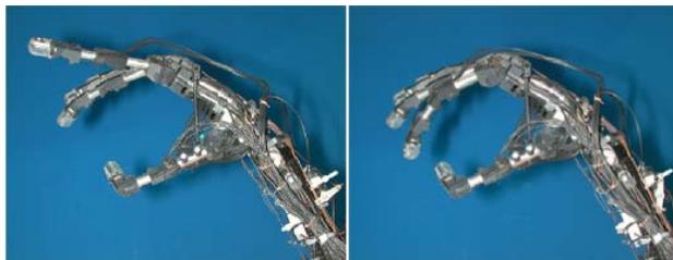
**FIGURE 7: Robotic hand** as a platform for EAP demonstration [This Robotic Hand is a courtesy of Graham Whiteley, Sheffield Hallam University, UK.; The actuators installed by Giovanni Pioggia – U. of Pisa, Italy/JPL (Photographed at JPL)]
