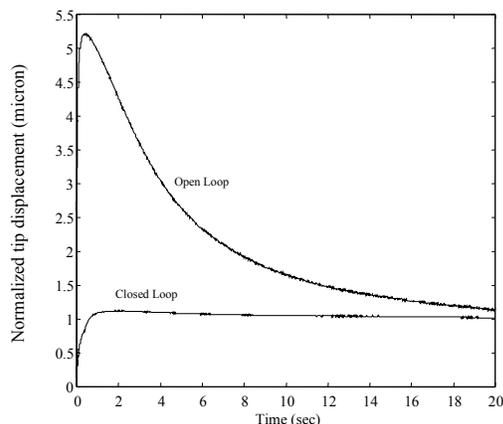
**FIGURE 16:** Comparison of open- and closed-loop step response for an ionic polymer actuator.
