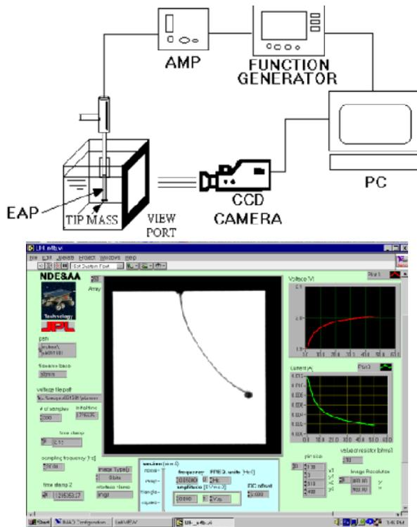
**FIGURE 9:** Displacement measurement setup and the display of the activated IPMC with tip mass.
