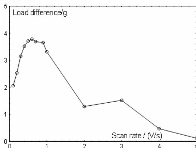
**FIGURE 3:** Maximum difference in measured load between oxidized and reduced states for 10 mm PPy (DBS) actuators as a function of scan rate (5 V/s corresponds to ~0.7 Hz). 0.1 M NaCl is the cycling electrolyte
