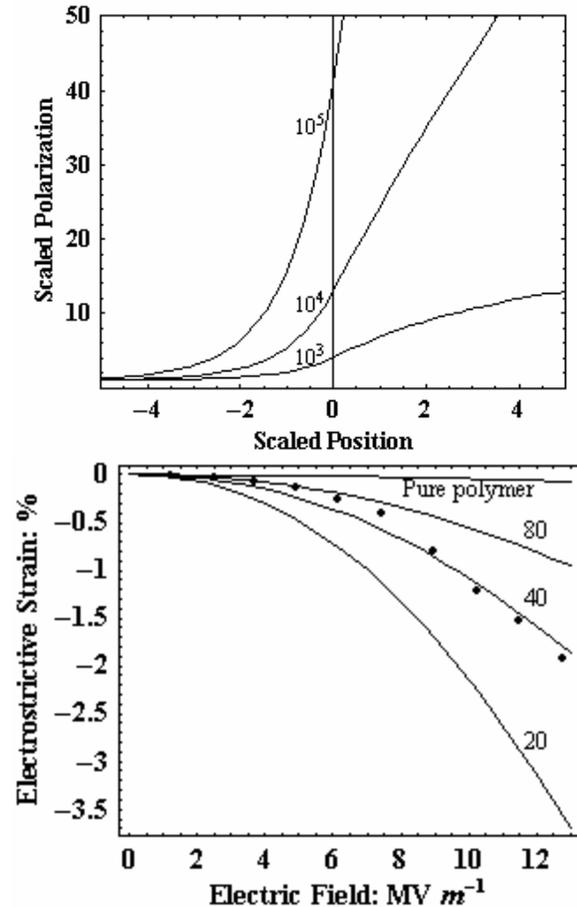
**FIGURE 13:** Top: the polarization profile at the composite interface for various dielectric constant of the second phase; Bottom: the strain versus electric field for various heterogeneity sizes of second phase.
