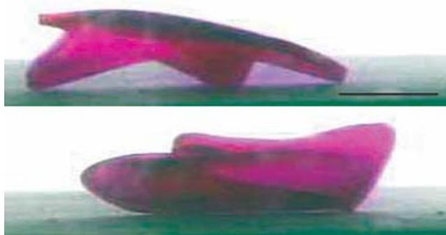
**FIGURE 4:** Starfish-shaped gel robot made of EAP that turns over: The scale bar is 5[mm]. Photos show gel robots 20 and 50[s] after applying the electric fields.
