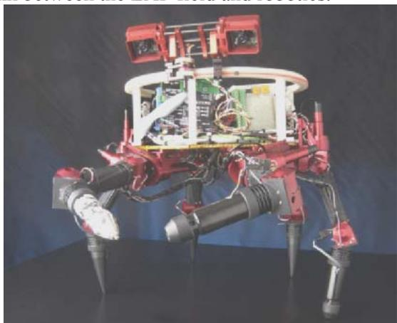
**FIGURE 9:** The JPL's LEMUR robot representing the new class of biomimetic robots that could be used as platforms for EPA to enhance these robots performance.
