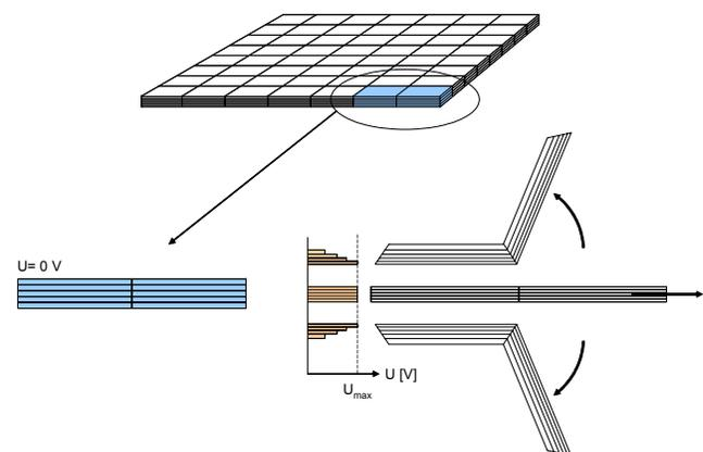
**FIGURE 8:** Concept of a large scale shell actuator for possible applications in lightweight structures.
