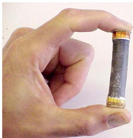
**FIGURE 10:** Multifunctional Electroelastomer Roll (MER) Spring Roll
