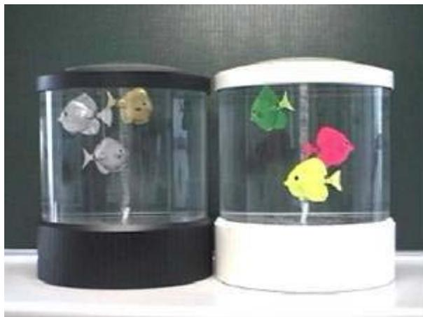
**FIGURE 1:** The first reported commercial EAP-based product in the form of a fish-robot. This fish is produced by Eamex, Japan.
