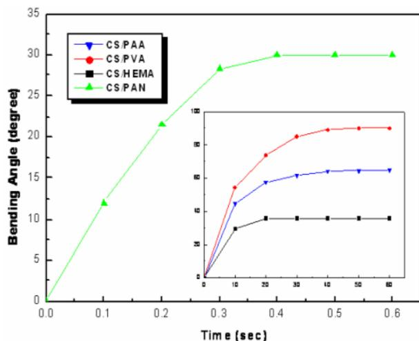
**FIGURE 6:** The bending angles of the hydrogels at a constant applied voltage (10 V) in a 0.8 wt% aqueous NaCl solution at 35 °C.
