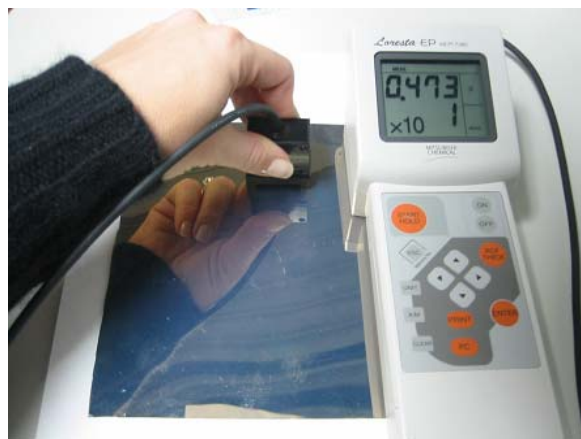
FIGURE 9: An example of the new self-assembled, low modulus, electrically conducting, nanostructured materials being tested.
