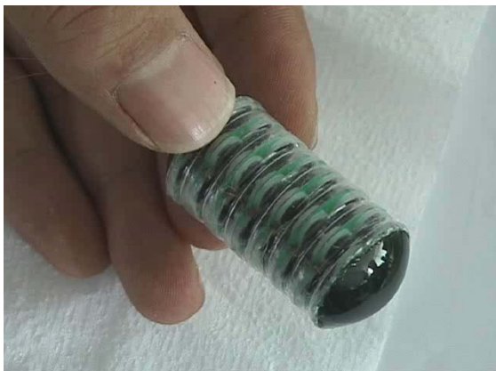
FIGURE 10: A tube-like smart pill that is a biomimetic moving mechanism.
