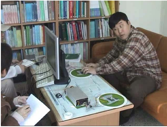
FIGURE 20: Evaluation of the EAP based Braille display device for the visually impaired.
