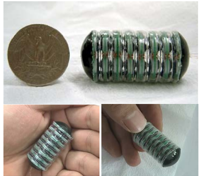
FIGURE 18: Different views of the smart pill that is a tube-like biomimetic moving mechanism.
