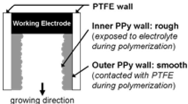
**FIGURE 15:** Schematic drawing of polymerization of PPy tubing.
