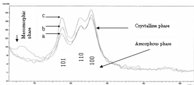
**FIGURE 31:** (a) X-ray diffraction pattern obtained from the non-irradiated PET microfiber keeping fiber axis parallel to x-ray beam, (b) x-ray diffraction pattern of proton irradiated microfiber keeping fiber axis perpendicular and (c) parallel to x-ray direction.
