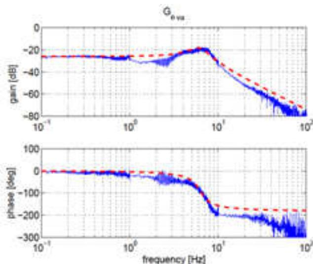
**FIGURE 34:** Frequency response from applied voltage to angle (solid: experimental, dashed: identified)
