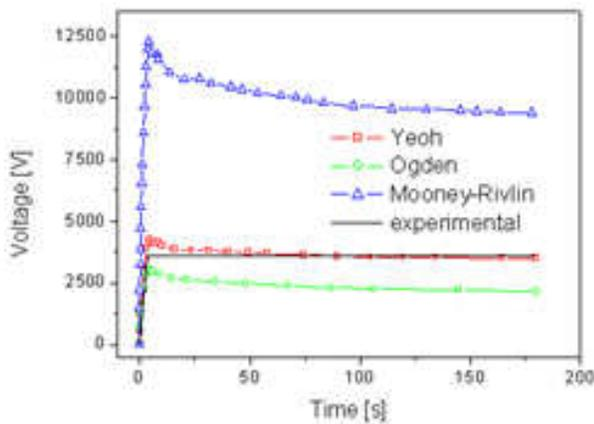
**FIGURE 22:** FE-calculation: time history of the voltage required to obtain the observed radial elongation history for the Yeoh-, Ogden- and Mooney-Rivlin-form.
