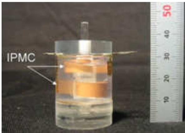
**FIGURE 32:** Rotary IPMC actuator
