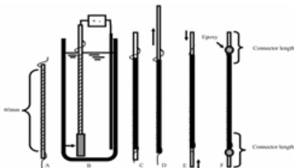
**FIGURE 3:** Method of preparing hollow tubes by electropolymerisation of pyrrole onto a helically wound platinum wire template. Removal of the inner platinum wire (step D) leaves a hollow tube in which a thinner platinum wire is contained within the PPy tube wall.
