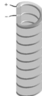
**FIGURE 11:** A new dielectric elastomer linear actuator.
