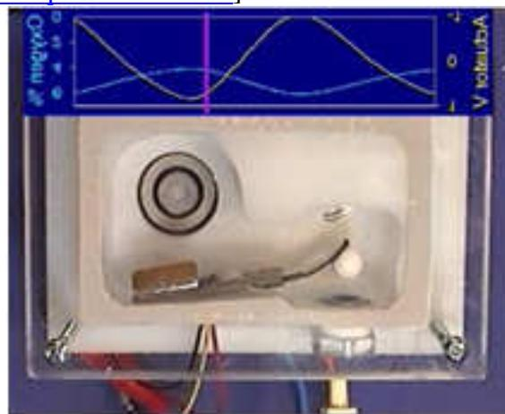
**FIGURE 6:** Open state of a bimorph actuator allowing air into a simulated apple box. The actuator was automatically opened when the oxygen sensor (top left) detected the oxygen content to be below the target state (5%).
