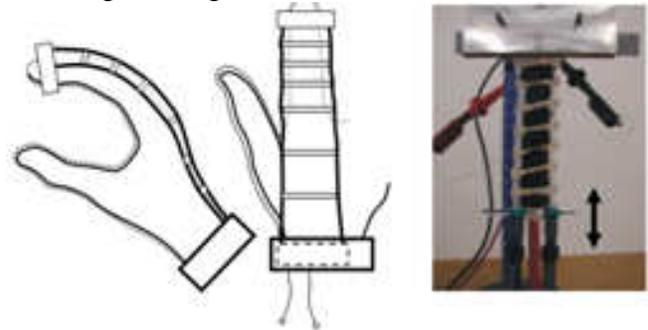
**FIGURE 23:** Schematic of a chain-like actuator (L.) and a demonstrator (R.)
