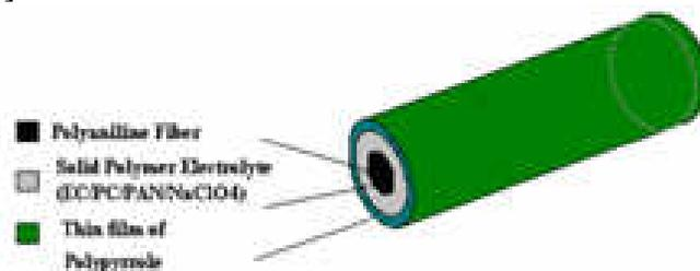
**FIGURE 8:** Scheme of a conducting polymer fiber actuator
