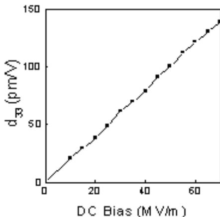
**FIGURE 20:** The apparent piezoelectric constant of the polymers under DC bias were characterized and a high piezoelectric constant was obtained
