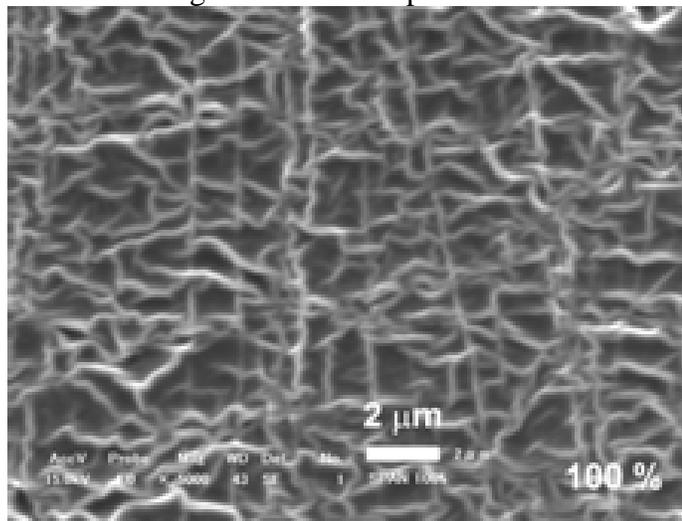
**FIGURE 17:** Scanning Electron Micrograph of PPy/PMAS film.
