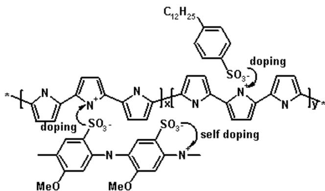
**FIGURE 18:** Scheme of electrochemical oxidation of PPy/(DBS/PMAS) film.
