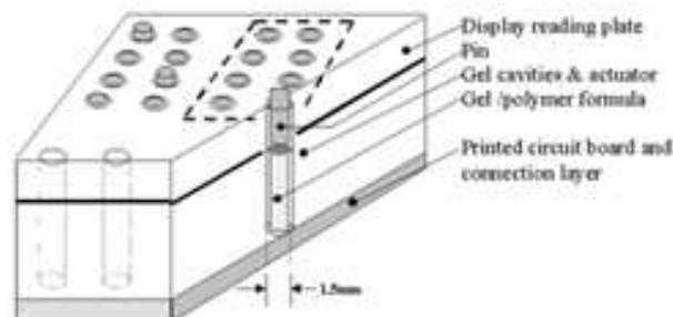
**FIGURE 5:** Design of an electronic Braille screen [[www.quantech.com.au](http://www.quantech.com.au)]
