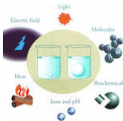
**FIGURE 7:** Stimuli enabling mechanical responses of polyelectrolyte gels.
