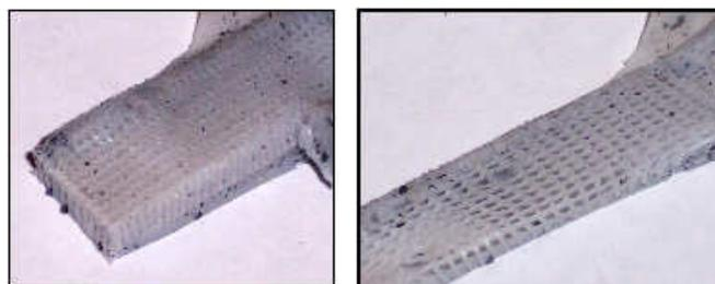
**FIGURE 25:** Rectangular celled SPEM made using rapid prototyping technology. Elongated state is on the right. The sample is 2 cm in width, 10 cm length, and .6 cm depth.
