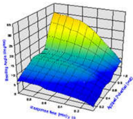
**FIGURE 29:** Plot of bending angle of actuators Vs. various backing layer thickness
