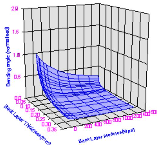
**FIGURE 28:** Plot of bending angle of actuators Vs. various backing layer thickness with modulus
