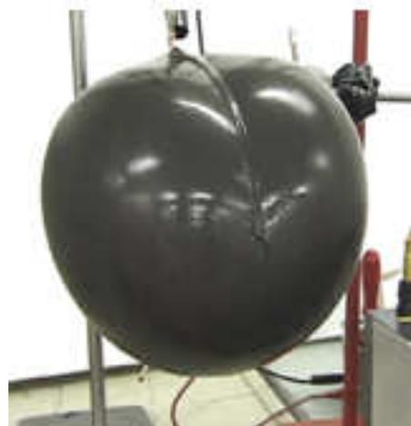
**FIGURE 24:** Passive (top) and activated (bottom) dielectric elastomer balloon actuator filled with air.
