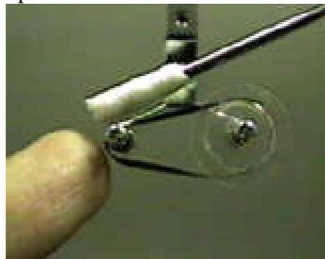
**FIGURE 16:** Polypyrrole motor transducers the free energy change of sorption directly into a continuous rotation.
