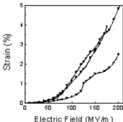
**FIGURE 19:** The electrostrictive strain response of some P(VDF-CTFE) copolymers
