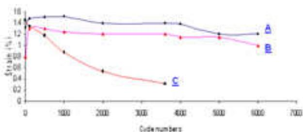
**FIGURE 4:** Actuator strain obtained from a PPy helix tube operated at 1Hz in 3 electrolytes: A and B are ionic liquids and C is a propylene carbonate based electrolyte.
