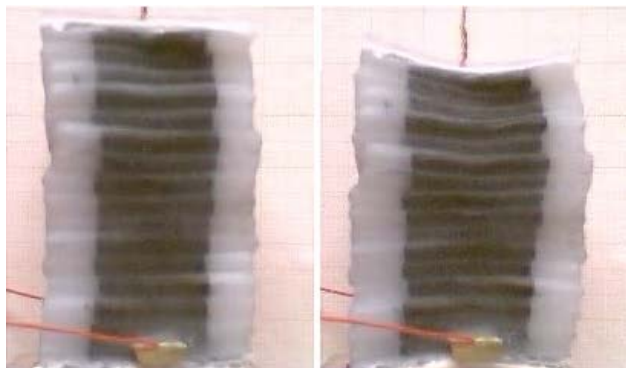
FIGURE 13: A 15% contraction of a prototype folded dielectric elastomer actuator.
