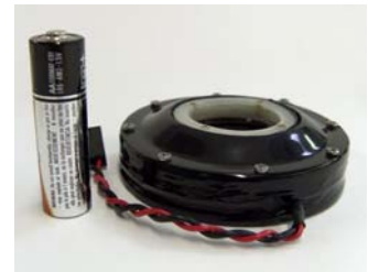
FIGURE 14: UMA Based Linear Actuator with Integrated Thunder Power Supply
