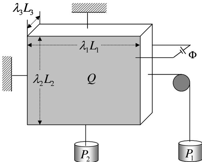
**FIGURE 9:** A layer of a dielectric elastomer coated with two compliant electrodes, and loaded by a battery and two weights.
