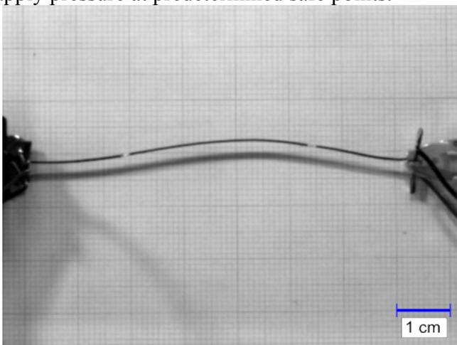
**FIGURE.5:** Bi-stable buckled beam
