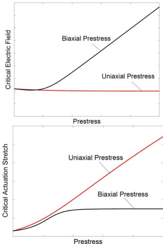
**FIGURE 10:** Electromechanical responses of dielectric Elastomer actuators subject to pre-stresses.
