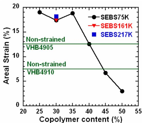
**FIGURE 11:** Maximum areal strain as a function of copolymer content of SEBS triblock of three different molecular weights under no-prestrain conditions.
