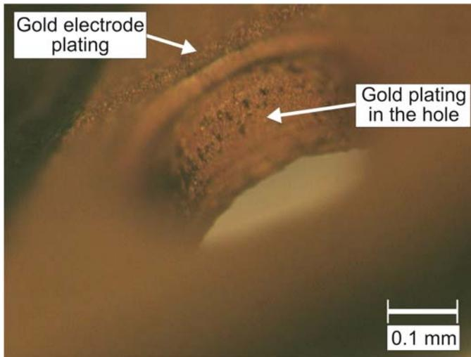
**FIGURE. 4:** Through-polymer connection
