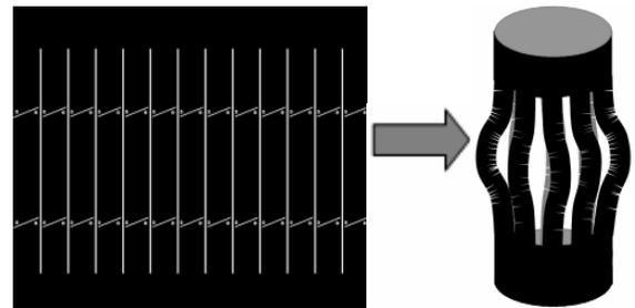
**FIGURE 7:** Concept of a linear actuator rolled-up from a single sheet.
