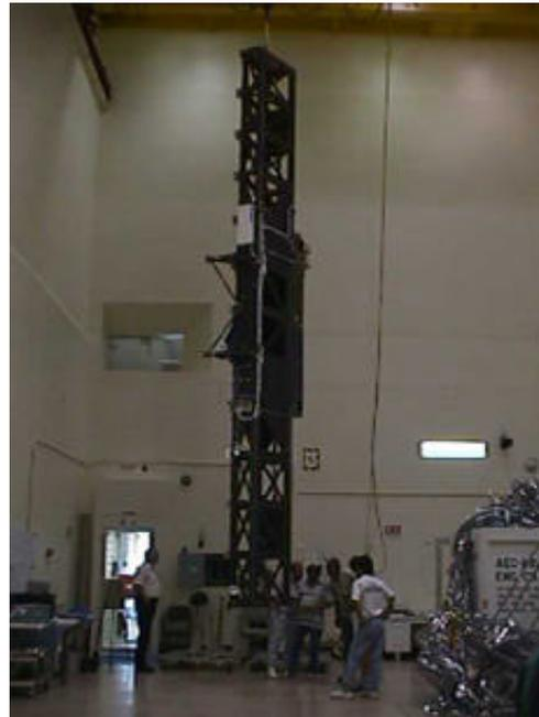
**Figure 4:** Outboard Support Structure (OSS) for the SRTM project, which consists of a graphite/epoxy structure.
