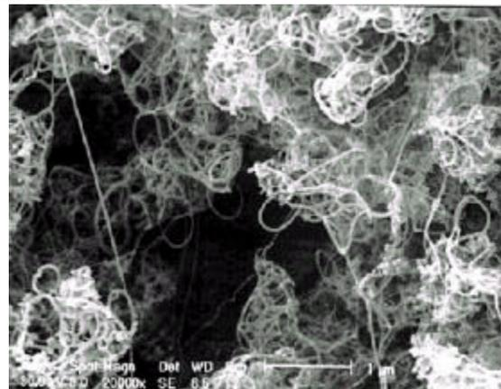
**Figure 9:** Bundles of carbon nanotubes, produced at JSC, as they appear before purification.
