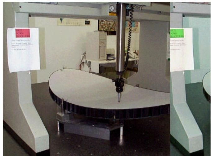
**Figure 3:** Coordinate Measuring Machine (CMM) checking the surface of the reflector.
