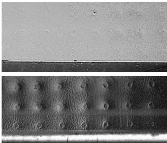
**Figure 10: Top** - Lap splice joint from a Boeing 727, as seen by the unaided eye. **Bottom** - EOL image of the same lap splice joint clearly showing corrosion pillowing.
