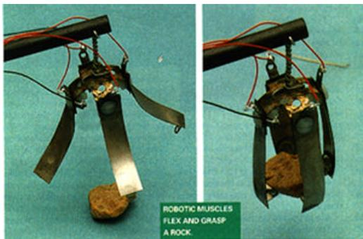
**Figure 8:** A gripper with electroactive polymer fingers for a miniature, light robotic arm.
