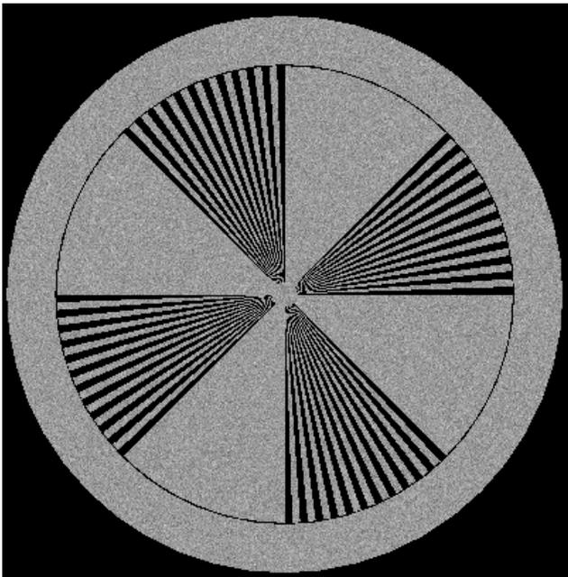
Simulated radiograph of a penetrometer gauge.
