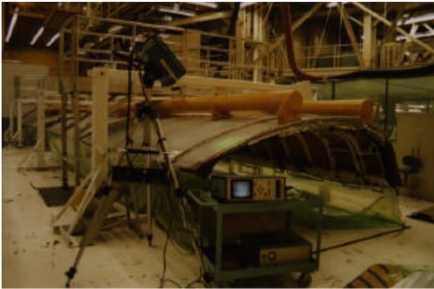
Tripod mounted shearography camera/laser is shown inspecting the aft end of PLBD #4 at location of delamination in a solid laminate frame member.
