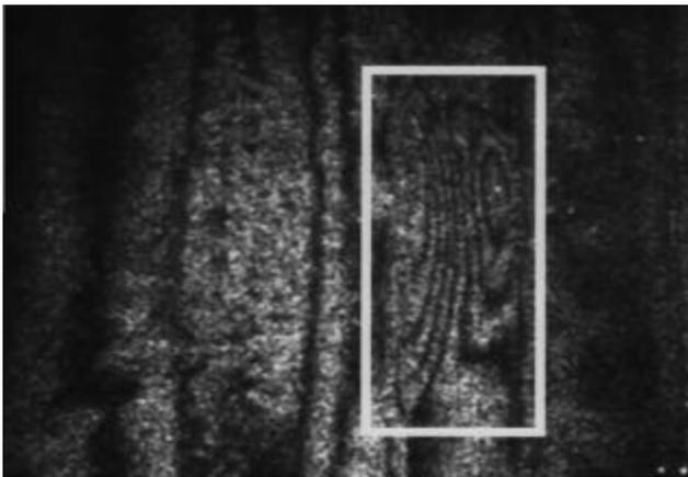
A view of a delamination (highlighted in the white frame) indication as seen on the image of processor. Flaw dimensions are 6.5x2.3 inches.
