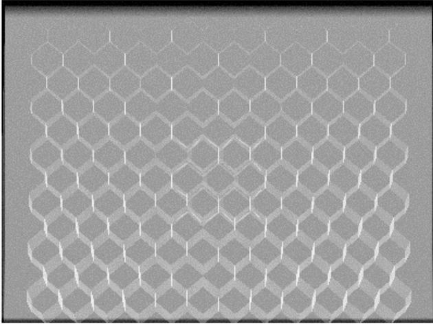
Simulated radiograph of a honeycomb sandwich using the CNDE developed computer code.
