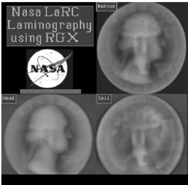
Reverse Geometry X-ray ® allows viewing different depth sections. Picture is showing different depths of a quarter coin.
