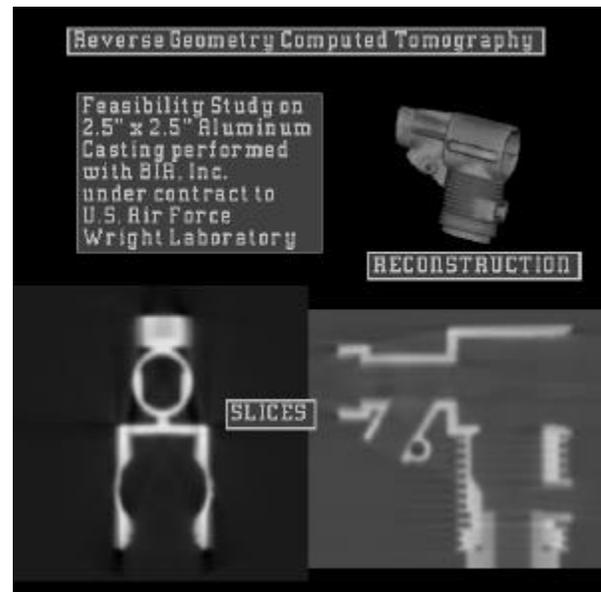
Reverse Geometry Computed tomography test of an aluminum casting showing various slices.
