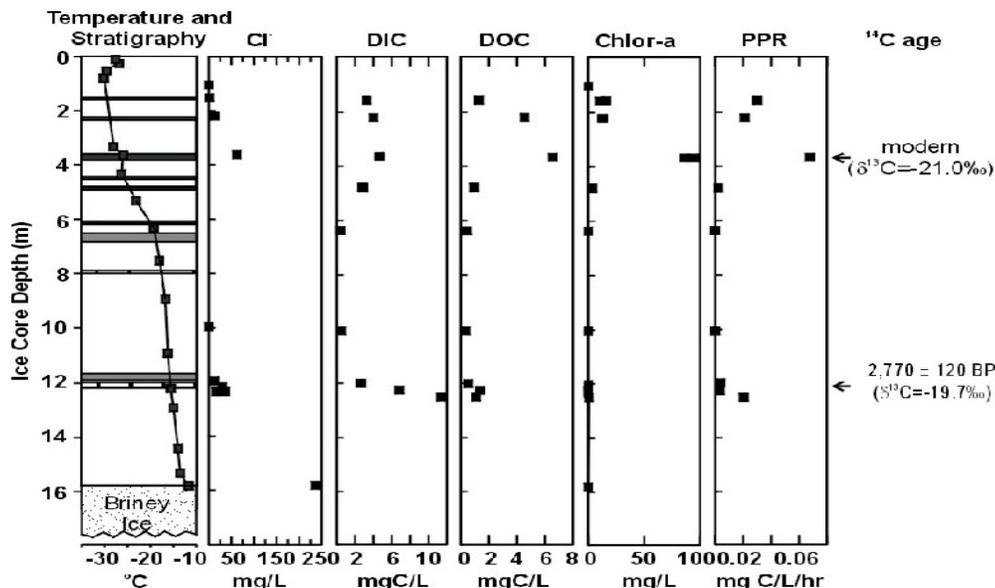
**FIGURE 5:** Physical and chemical properties of Lake Vida ice core taken in October 1996. Black horizons on the stratigraphy plot represent sediment layers, gray horizons are sandy ice, and vertically banded horizons contain microbial mat. The temperature profile shown was taken at the time of ice extraction.
