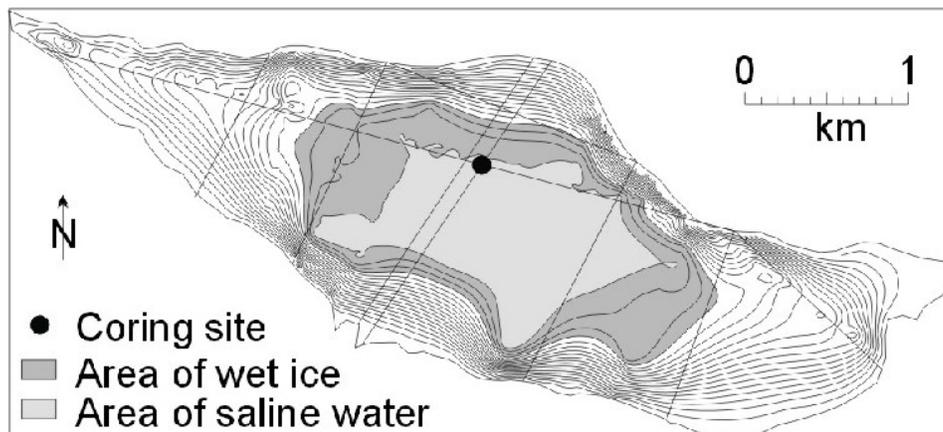
**Figure 4:** Bathymetric map of Lake Vida based on GPR and ice coring. GPR transect lines are shown. Solid black circle is the coring site.
