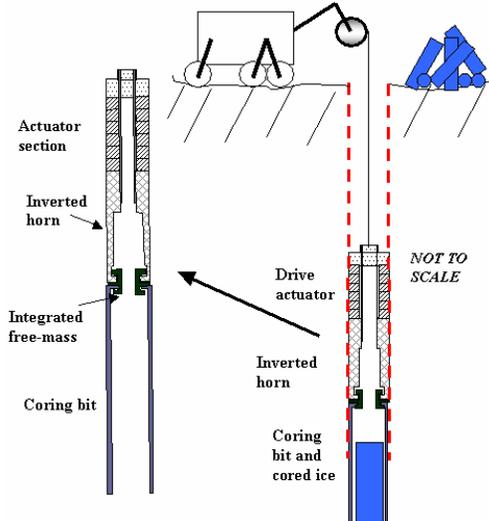
**FIGURE 6:** Schematic view of the ultrasonic-gopher operating inside the borehole.
