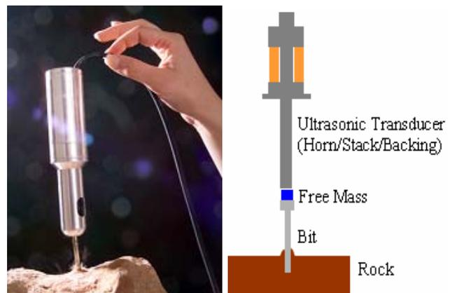
**FIGURE 3:** A photographic view of a prototype Ultrasonic/Sonic Gopher that drilled limestone and the core that was created.
