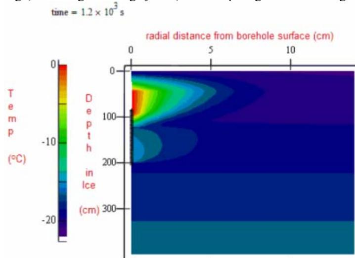
**FIGURE 8:** Thermal model results at 20 minutes indicating further melting near the piezoelectric stack but no melting at the bit/ice interface.
