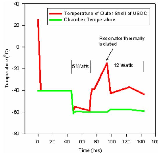
**FIGURE 7:** Tests of the USDC operation at low temperatures (conducted at the JPL's Extraterrestrial Materials Simulation Laboratory)
