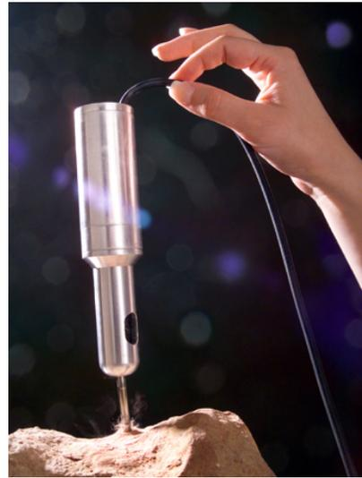
Figure 2. Ultrasonic/Sonic Driller/Corer (USDC) in action.
