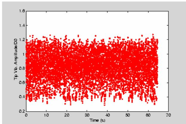
Figure 8. Horn vibration amplitude normalized by the amplitude without loading.
