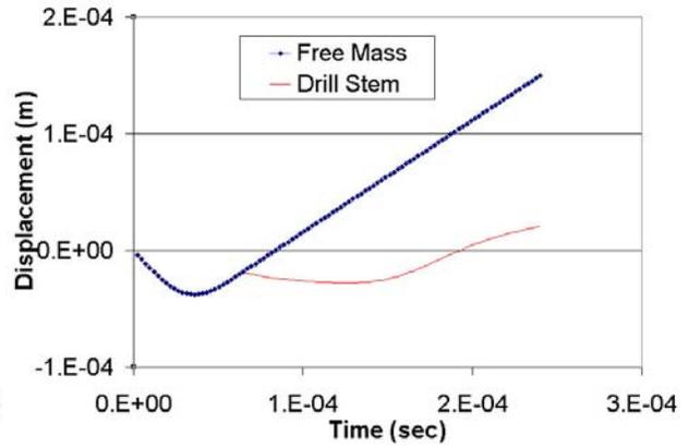
Figure 6. The free mass and drill stem displacement as a function of time.
