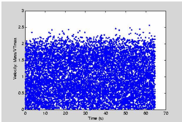
Figure 7. Free-mass velocity normalized by the horn tip vibration velocity.
