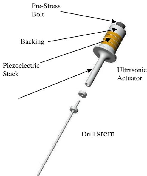
Figure 1. Exploded view of a typical USDC.
