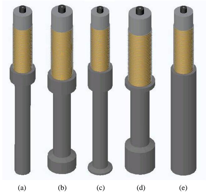
Figure 4. The 5 designs of ultrasonic horn studied:
