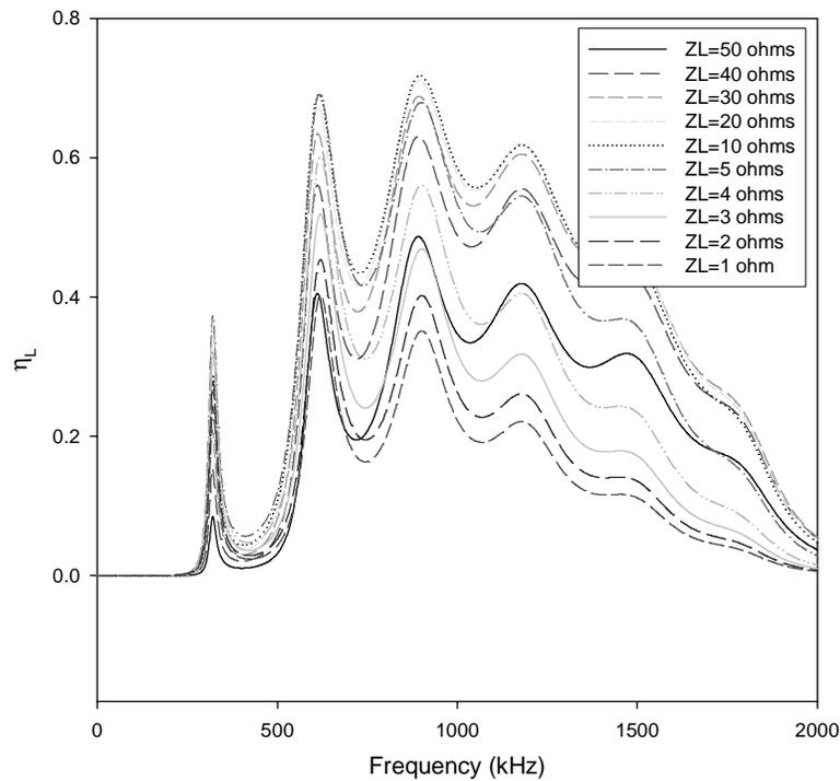
**Figure 8.** The efficiency as a function of the load impedance for the acoustic electric transformer using the measured material constants shown in Table 4.
