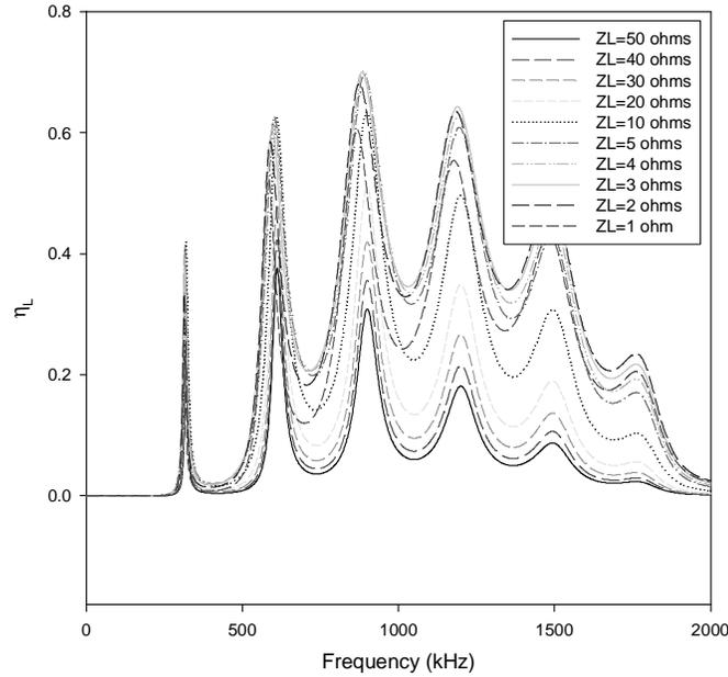
**Figure 6:** The efficiency for the acoustic electric transformer using the measured material constants shown in Table 3.
