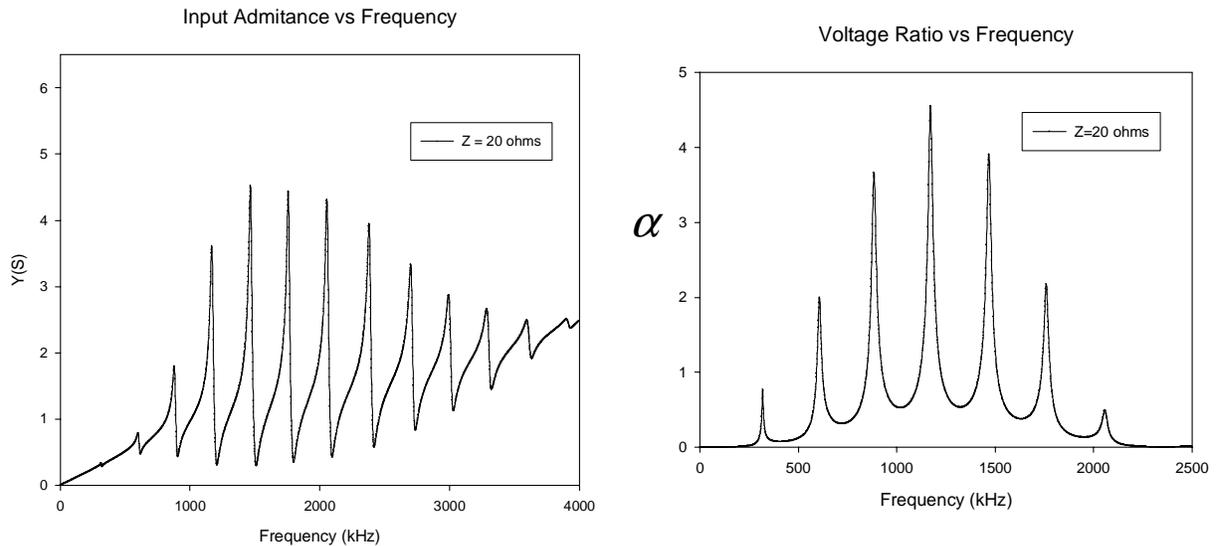
**Figure 5.** Input admittance and voltage ratio of the device with measured material constants shown in Table 3. The output piezoelectric is shunted by a 20 ohm load impedance.
