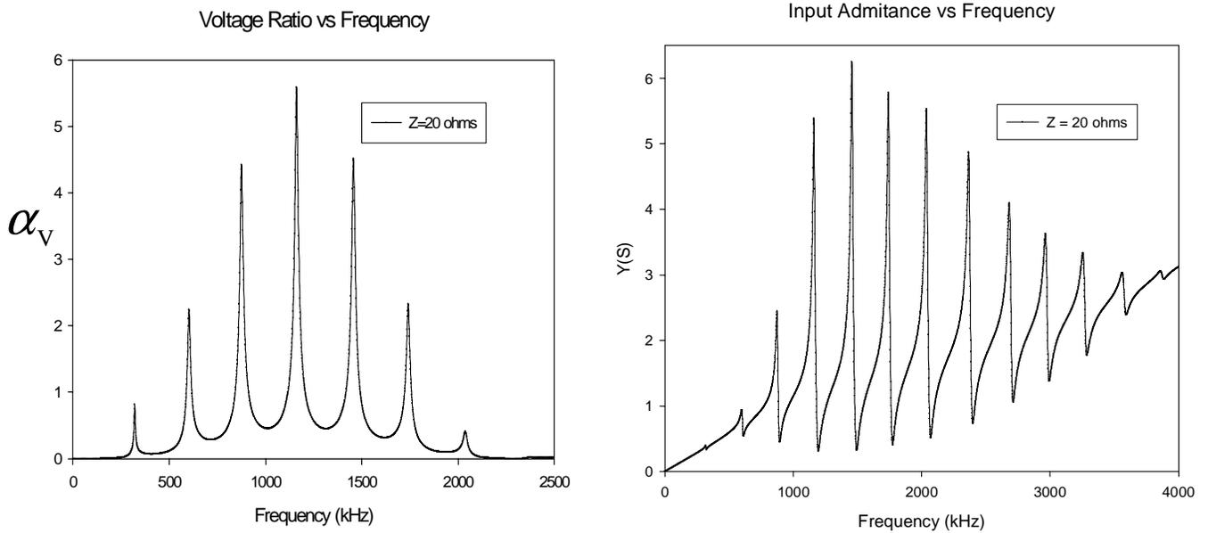
**Figure 3.** The voltage ratio and input impedance based on the input data and geometry published by Hu et al.<sup>1</sup> using the electromechanical model discussed in this paper. The curves are identical to data that was published by Hu et al. which was based on solving the wave equation directly.
