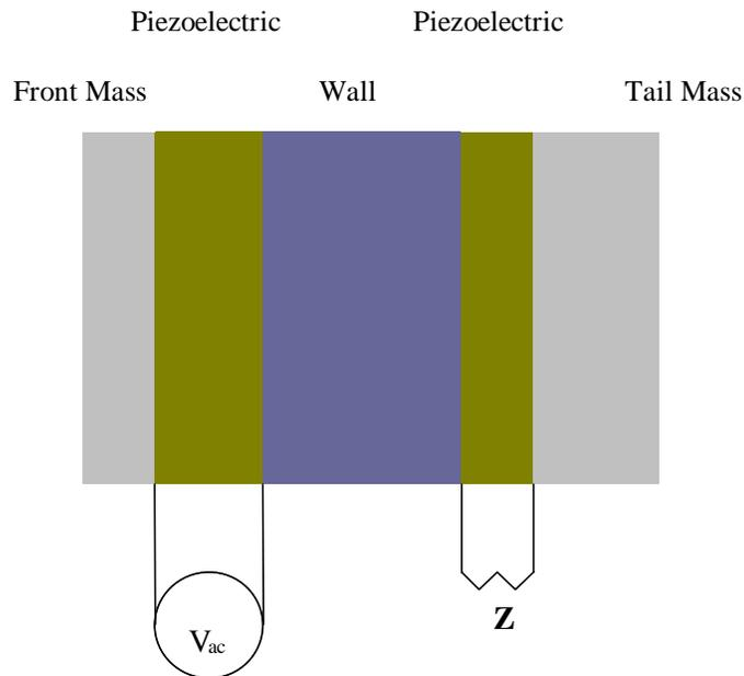
**Figure 1.** Schematic of the physical acoustic-electric system with a piezoelectric generator and receiver. The tail and front mass are optional. The delivered power is consumed in the impedance  $Z$
