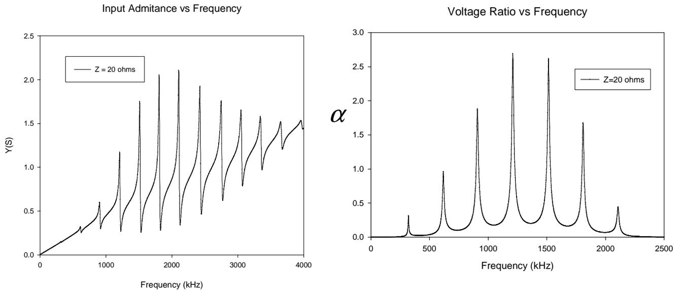
**Figure 7.** Input admittance and voltage ratio of the device with measured material constants (PZT-8) shown in Table 4. The output piezoelectric is shunted by a 20 ohm load impedance.
