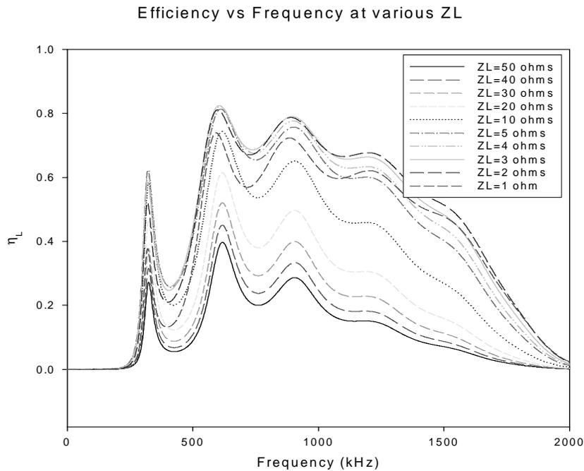
**Figure 4.** The efficiency of the power transfer for the acoustic electric feed-through described by Hu et al.<sup>1</sup> as a function of the frequency. Maximum efficiency is about 82.5% at  $Z_L=3$  ohms at 650kHz.
