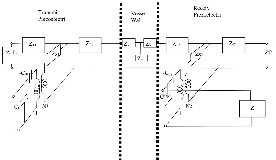
**Figure 2.** Schematic of the network equivalent circuit for the physical system shown in Figure 1. The delivered power is consumed in the impedance  $Z$ .  $Z_{TL}$  and  $Z_{TR}$  are the terminating mechanical impedances associated with the front and tail mass.
