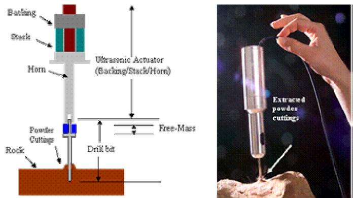
Figure 1. Photograph and Schematic of the Ultrasonic/Sonic Driller/Corer.
