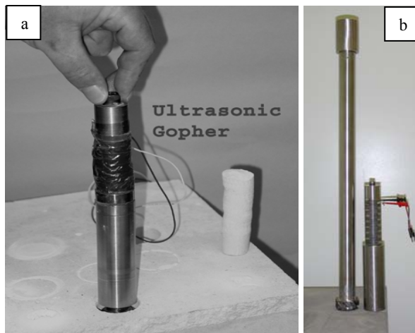
Figure 3: a) Ultrasonic-Gopher and extracted limestone core, b) Recent prototype of ice gopher. Ice chisel bit on the left and actuator on the right.
