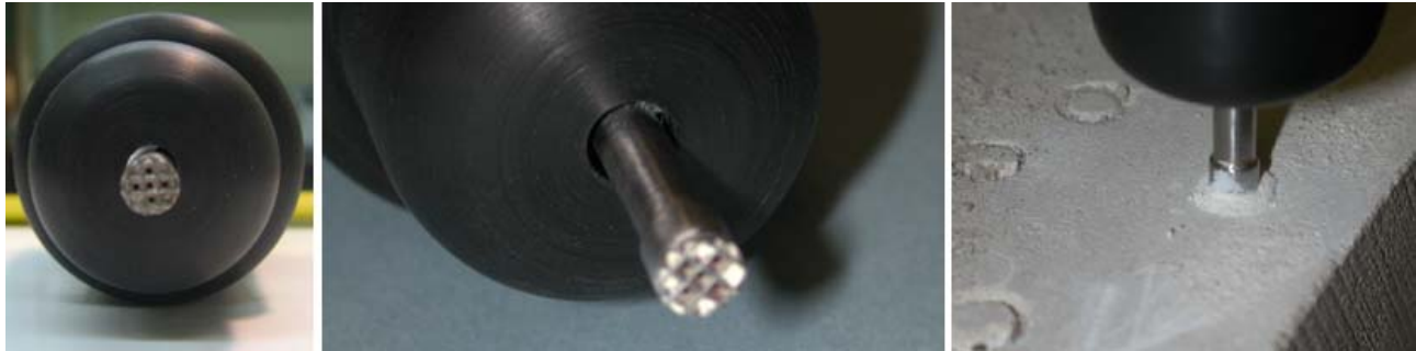
FIGURE 12: Various photographic views of the bit: Left: bit bottom with the holes; Middle: Side view; and Right: The bit drilling limestone.
