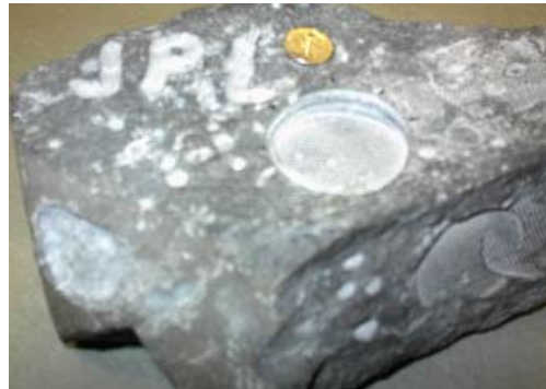
FIGURE 10: Photographic view of a basalt that was abraded by the URAT. The footprint of the abrasion bit can be seen on the surface.
