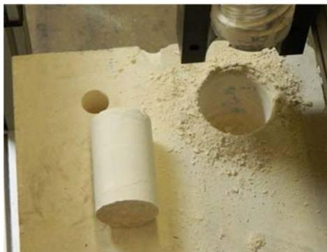
**Figure 6:** The recovered core samples were 57 mm diameter and 100 mm long. The cores recovery was 100% successful.
