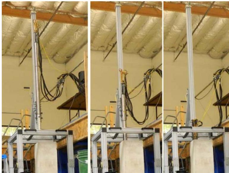
**Figure 5:** Drilling progress into 2 meter high limestone column.
