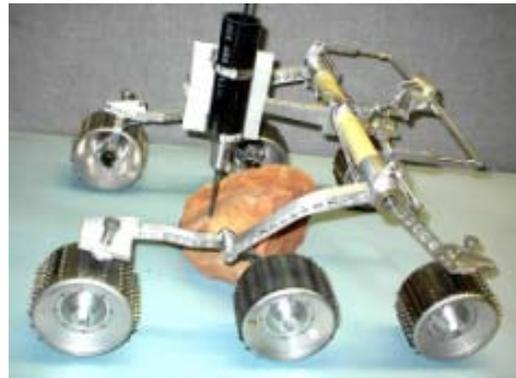
**FIGURE 7:** The USDC mounted on the Sojourner Rover platform is shown to drill sandstone.
