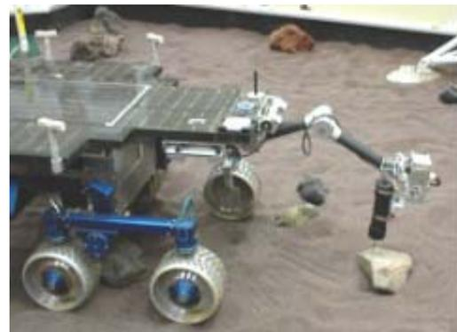
**FIGURE 8:** The USDC is shown drilling while mounted on the robotic arm of the FIDO Rover.
