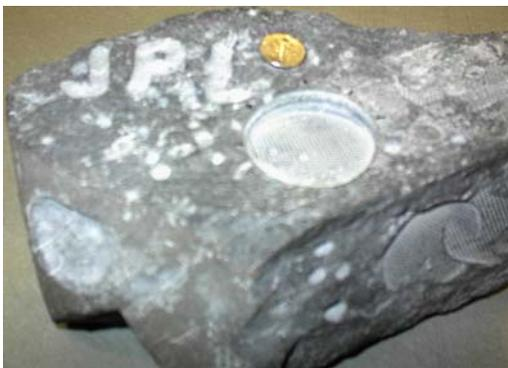
**FIGURE 4:** Basalt rock sample abraded by the ultrasonic rock abrasion tool.
