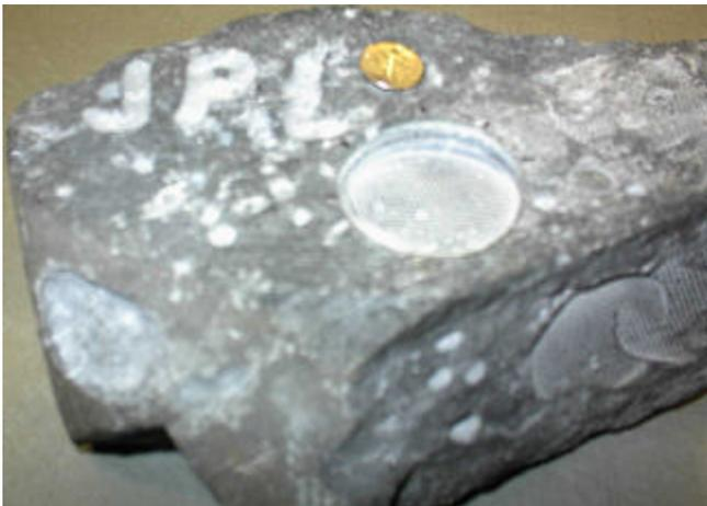
Figure 13. Basalt rock sample tested using the abrasion tools shown in Figure 11.
