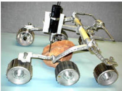
Figure 16. Coring from a Sojourner class rover.
