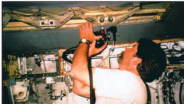
Figure 2: A view of the application of MAUS and the hand-held probe in a field test.
