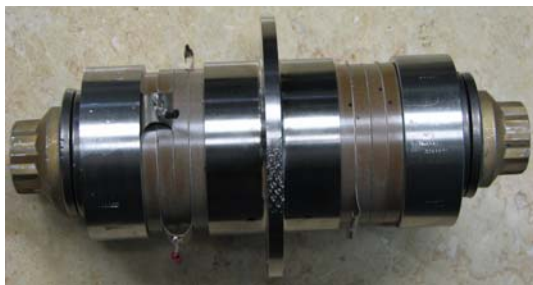
Figure 13. A photograph of a high power acoustic electric feed-through prototype. The final design had six piezoelectric rings.
