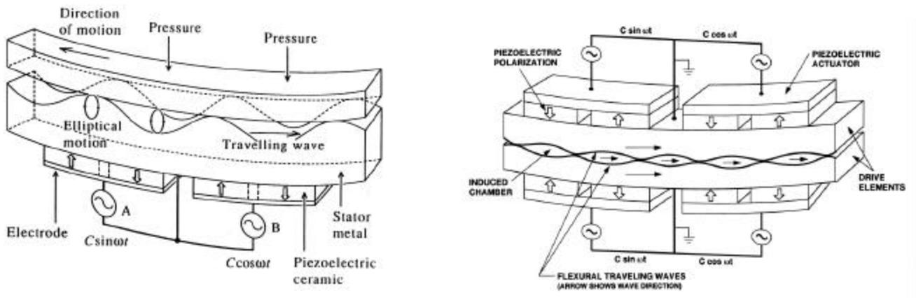
**FIGURE 1:** Principle of operation of a piezoelectric motor.
