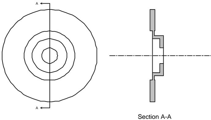
**Figure 7:** Metal ring of the piezo pump.
