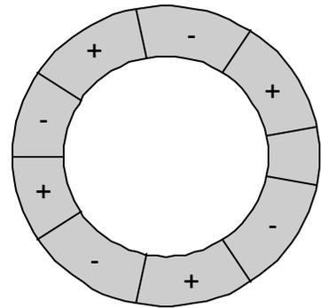
**Figure 8:** A piezoelectric ring designed for 4-wave mode.
