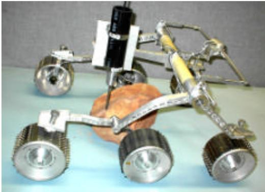
**FIGURE 14:** The USDC mounted on the Sojourner Rover platform is shown to drill sandstone.
