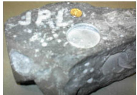
**FIGURE 13.** Basalt rock sample tested using the abrasion tools.
