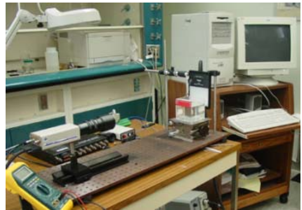
FIGURE 1: Setup for data acquisition of the curvature as a function of various parameters for IPMC.
