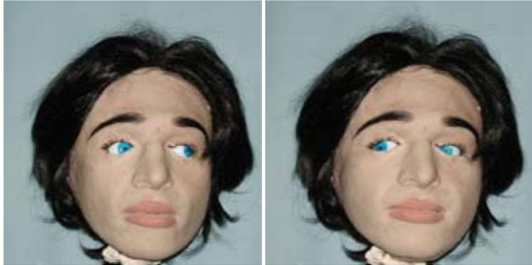
**FIGURE 8:** An android head (Photographed at JPL) as EAP platform will use such actuators to make facial expressions (Courtesy of G. Pioggia, University of Pisa, Italy).
