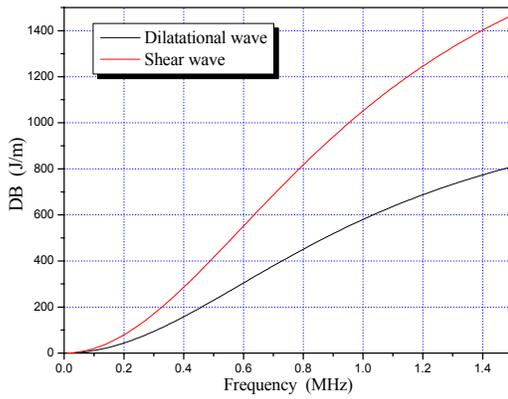
Fig. 9: Energy dissipation in the biomaterial as a function of frequency.
