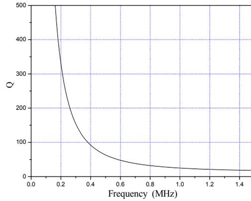
Fig. 10: Attenuation factor,  $Q$ , as a function of frequency in the biomaterial
