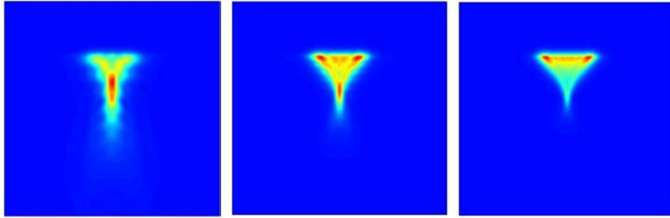
Fig.12: Temperature distributions in the biomaterial at 8 sec. 0.5 MHz (left panel), 1 MHz (middle panel) and 1.5MHz (right panel)
