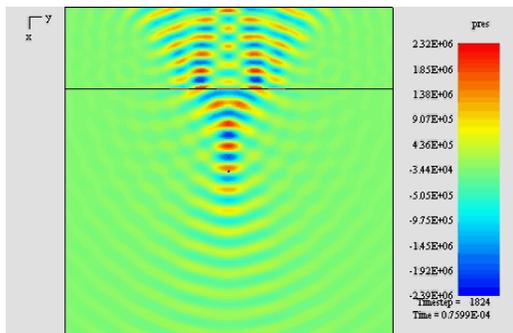
(a) Steady pressure field produced by a continuous wave.
