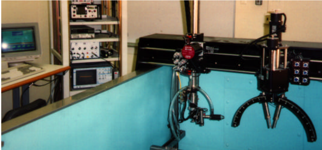
FIGURE 1: A view of the LLW scanner (on the right portion of the bridge) installed on the JPL's C-scan system
