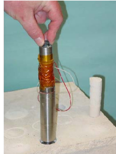
FIGURE 6: An Ultrasonic-Gopher and an extracted core (right) from a limestone.
