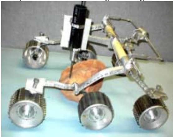
FIGURE 8: The USDC mounted on the Sojourner Rover platform is shown to drill sandstone.
