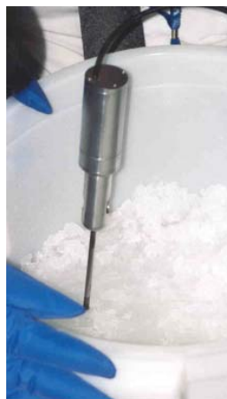
FIGURE 7: Tests of the USDC operation at low temperatures (conducted at the JPL's Extra-terrestrial Materials Simulation
