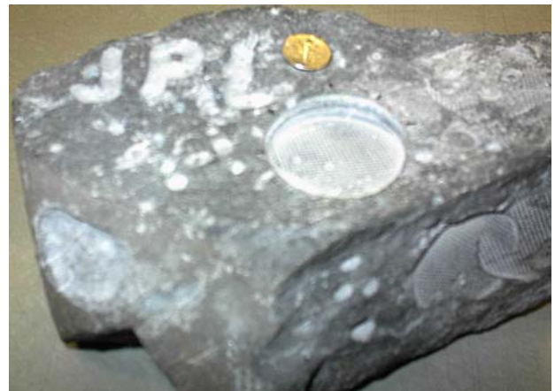
FIGURE 5: Basalt rock sample abraded by the ultrasonic rock abrasion tool.
