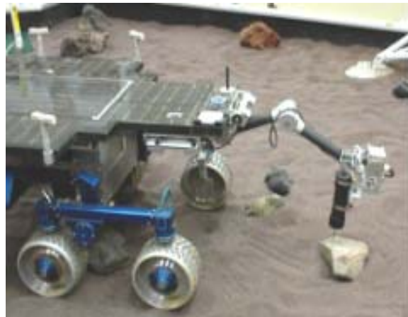
FIGURE 9: The USDC is shown drilling while mounted on the robotic arm of the FIDO Rover.
