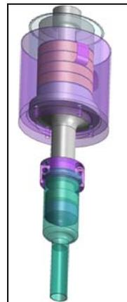
**Figure 4:** The in-and-out anchoring USDC.
