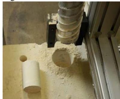
**Figure 8:** Using the Auto-Gopher, the first core (57.25 mm diam. and 97.25 mm long) that was produced of limestone (Photo courtesy K. Zacny, Honeybee Robotics).
