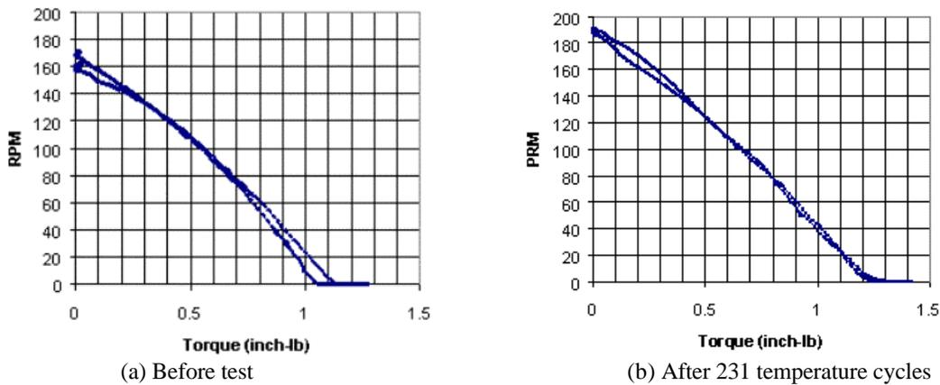
Figure 7: Temperature cyclic test
